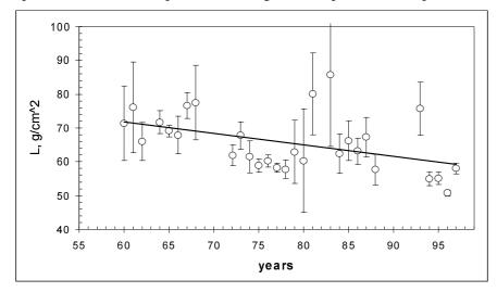
Fig. 2. The time dependence of *L* calculated from the absorption curves of the half-year averages of dN(x). The straight line shows the gradual decrease of *L*. The vertical bars give the values of standard errors.
