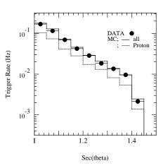
Fig. 3: Zenith angle dependence of the trigger rate under any four fold coincidence in the detectors. Each of any four detectors records a signal more than 1.25 particles. Simulation results are compared with the data. Solid and dashed lines show all primary particles and primary protons, respectively.
