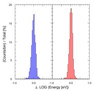
**Figure 1:** Accuracy of event reconstruction. Fluctuation of energy determination for  $3 \times 10^{19}$  eV (left) and  $10^{20}$  eV (right) showers with zenith angles less than  $45^{\circ}$ .
