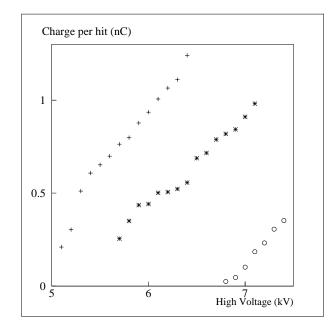
Figure 1: Detection efficiency of one RPC of the auxiliary telescope vs operating voltage for 3 gases: TFE/Ar/i-But=45/45/10 (+); 60/17/13 (\*) and 75/15/10 ( $\circ$ )
