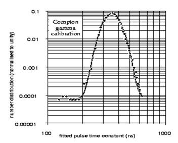
**Figure 3:** Time constant distributions (normalised to unity) for 5 kg NaI crystal: (*uppergraph*). Background distribution showing additional population of shorter pulses; (*lowergraph*). Compton calibration with <sup>60</sup>Co source (5 hours each day).
