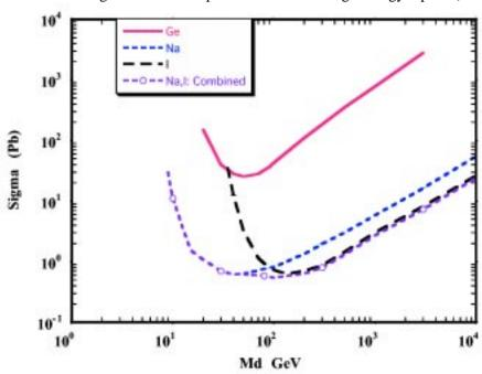
sis. Figure 1: Dark matter cross section limits in picobarns, corrected to the equivalent There is so far no explanation of proton cross section, as a function of LSP mass for the combined data
