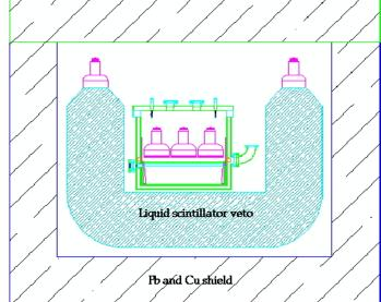
Figure 5: Two-phase ZEPLIN detector in scintillator veto
