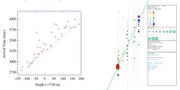
Figure 4: Event 1197960. Left: The recorded arrival times of photons are plotted versus the depth of the observing sensors. The slope of the dashed line is the result of the reconstructed zenith angle of 155°. Right: Neutrino candidate event in the 10 string array. The shading (size) of the data represents time (amplitude) of triggered photomultipliers. The reconstructed muon track moves upward over more than 300 m.
