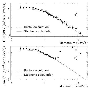
**Figure 1:** The flux (full circles) at float (3.9 g/cm<sup>2</sup> residual atmosphere) as a function of momentum for a)  $\mu^-$ , b)  $\mu^+$ . The open squares show  $\mu^-$  data from the MASS89 (Brunetti et al. 1996) experiment. The calculated values are from the Bartol group (Gaisser et al. 1995) and from Stephens (1981).
