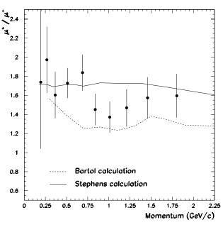
**Figure 2:** The  $\mu^+/\mu^-$  ratio at float (3.9 g/cm<sup>2</sup> residual atmosphere) as a function of momentum. The calculated values are from the Bartol group (Gaisser et al. 1995) and from Stephens (1981).
