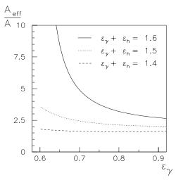
Figure 4: The enhancement in the gamma ray sensitivity, as a function of  $\epsilon_{\gamma}$ , for three different values of the global identification power of the network: 80% (full line), 75% (dotted line) and 70% (dashed line).
