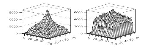
Figure 1: The hits distribution in the detector, for vertical events with the core at the centre of the carpet, for gamma (left) and protons (rights). Data are averaged over all the generated events.
