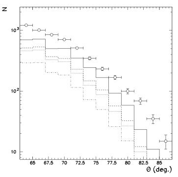
Figure 2: Simulated rate as a function of zenith angle compared to data. Broken curves illustrate the effects of different contributions to the rate. The bottom line is the contribution due to muon track length only and curves going upwards show the effect of adding  $\delta$ -rays, pair production and bremsstrahlung, and direct light on the PMTs. Proton primaries are assumed.
