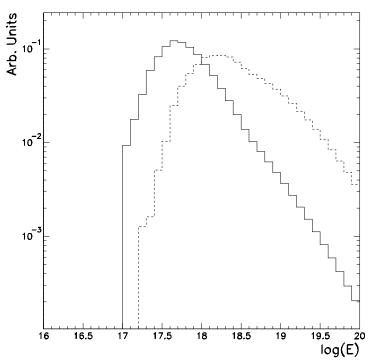
Figure 3: Energy response of the Haverah Park array to inclined showers for zenith angle  $70^{\circ}$  (continuous line) and  $80^{\circ}$  (dashed line).
