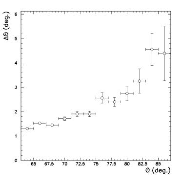
Figure 1: Zenith angle uncertainty as a function of zenith angle for inclined showers measured in the Haverah Park array.
