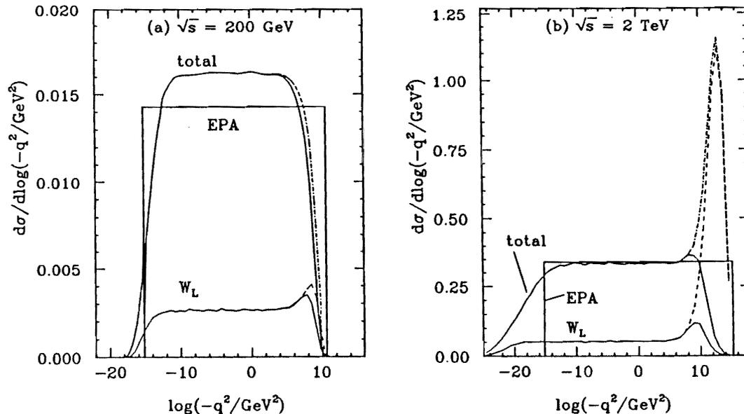
Fig.3  $\ln q^2$ -distributions for  $e^+e^-$  c.m. energies 200 GeV and 2 TeV. The solid box in each figure expresses the EPA estimation, and the dashed lines the contributions only from the diagrams with t-channel photon exchanges.  $W_L$  and ‘total’ mean the longitudinal W boson only and the sum of all the W boson helicity states, respectively.
