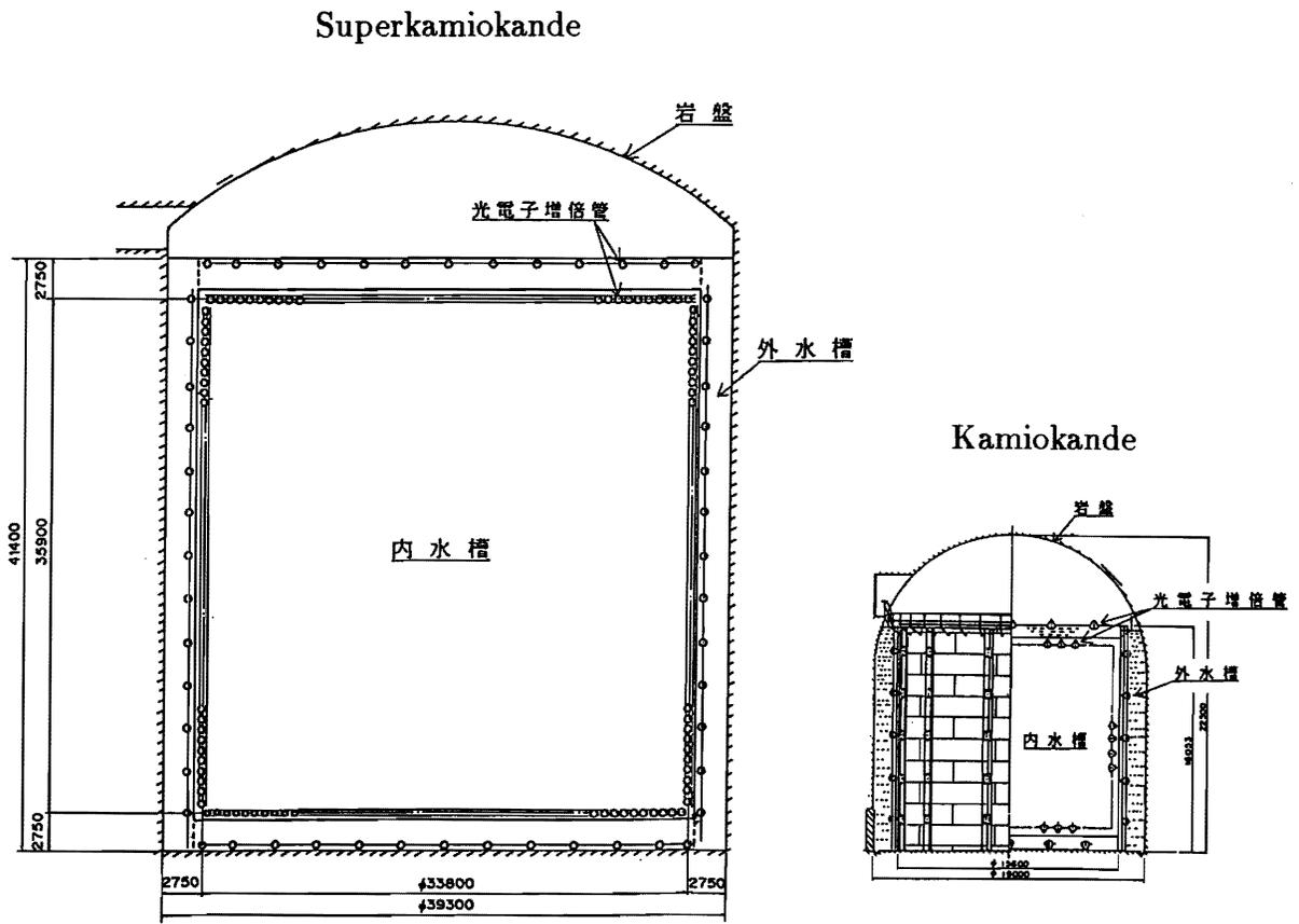
*Fig. 1. Comparison of the present Kamiokande detector and the proposed Superkamiokande detector.*
