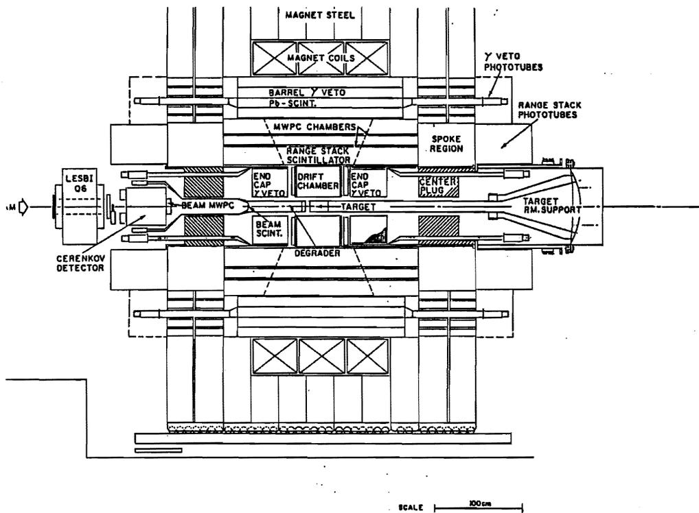
Fig. 4. Apparatus of BNL-E787 search for the  $K^+ \rightarrow \pi^+ \nu \bar{\nu}$ .
