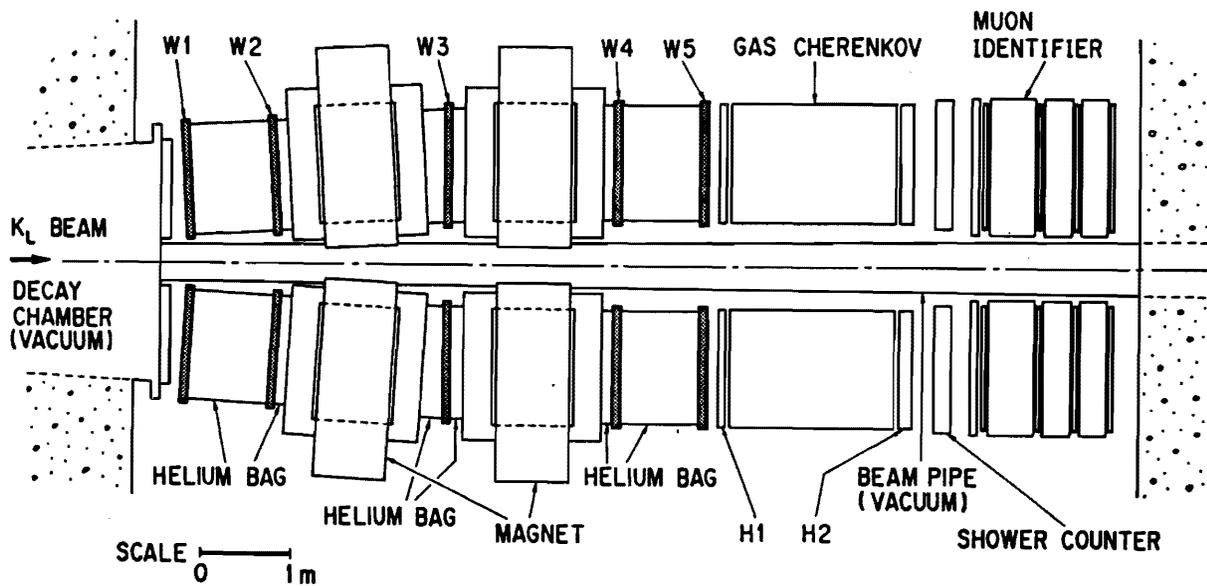
Fig. 1. Apparatus of KEK-E137 search for the  $K_L^0 \rightarrow \mu e$ .
