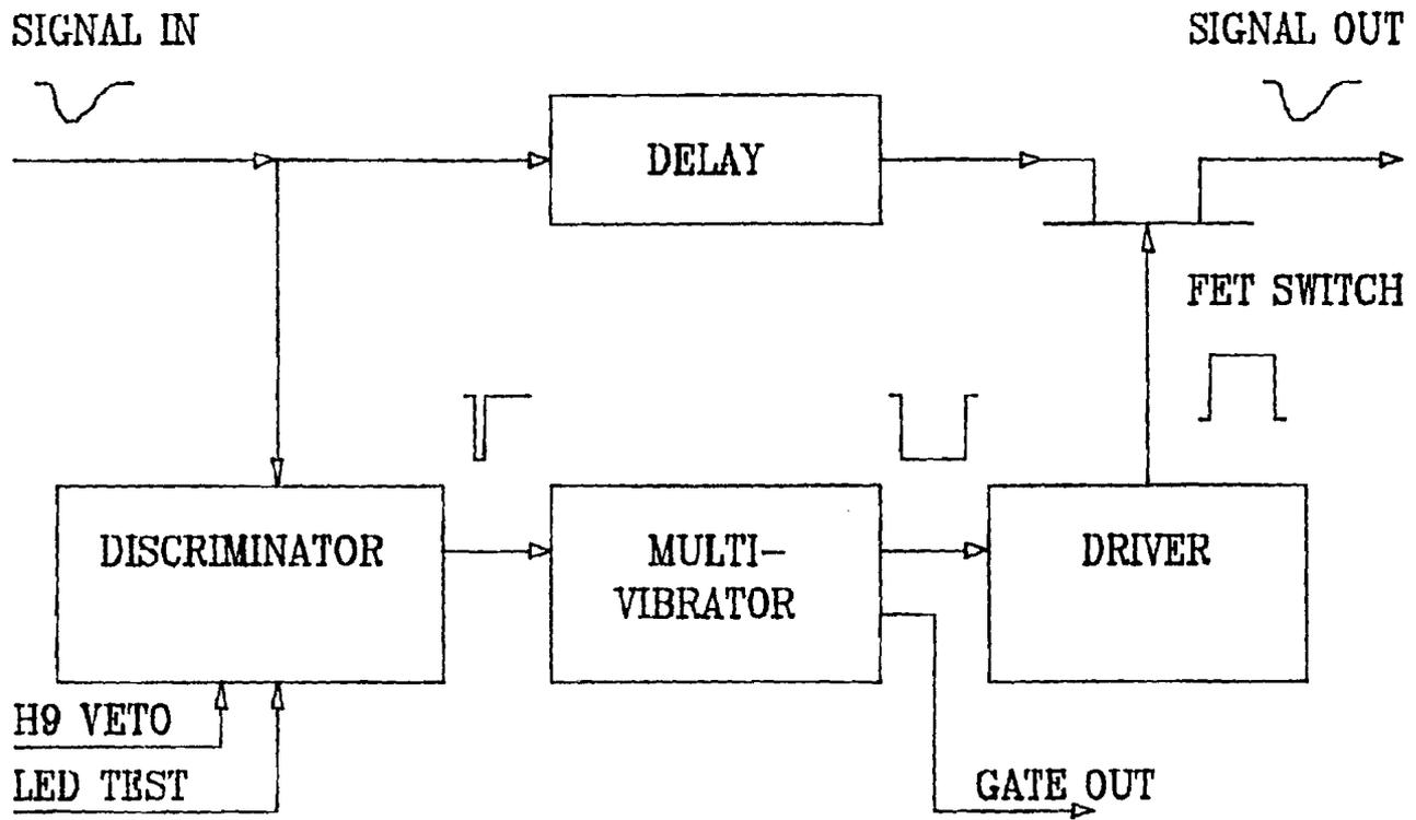
FIG. 2 ANALOG GATE LOGIC
