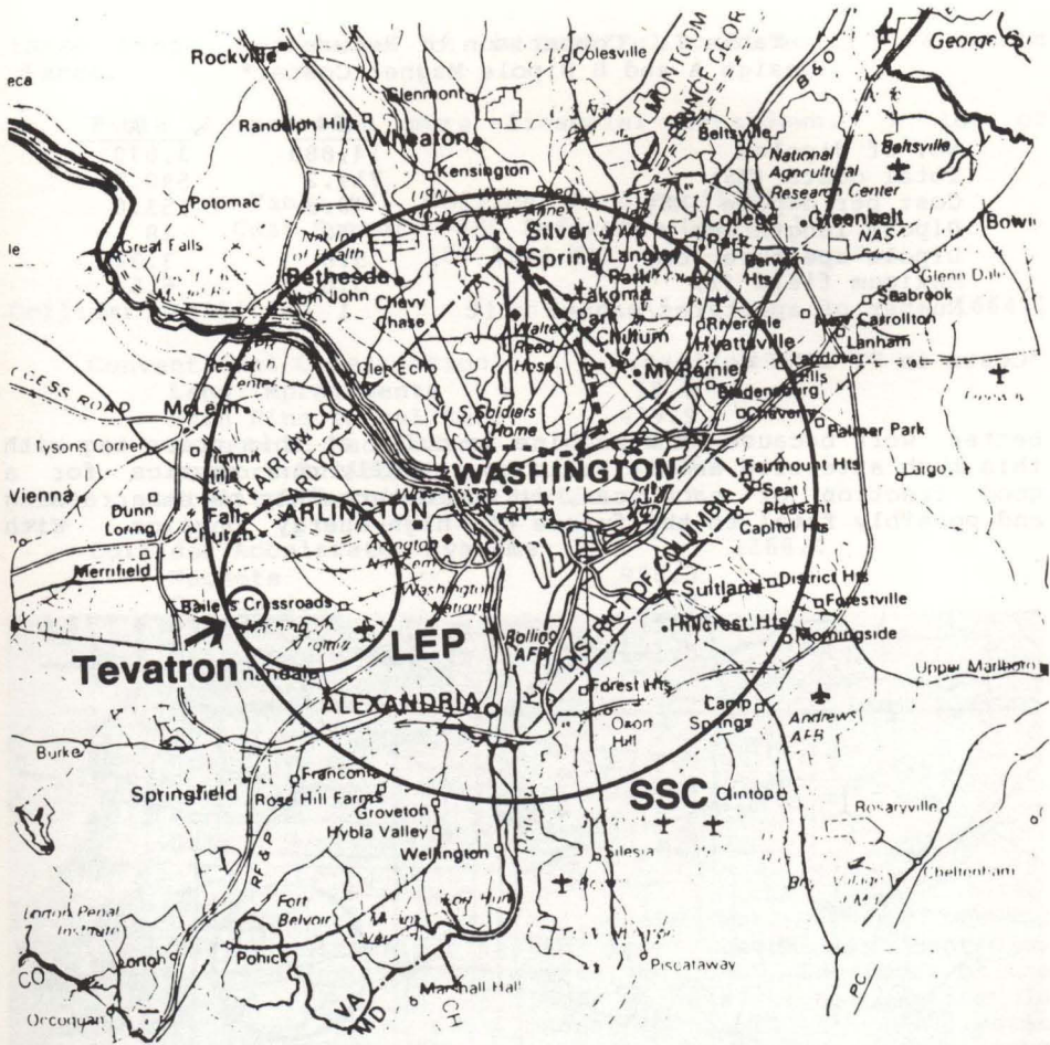
Fig. 4. The smallest diameter version of the SSC along with two smaller colliders, LEP at CERN and the Tevatron at Fermilab, superimposed to scale on the environs of Washington, D.C.
