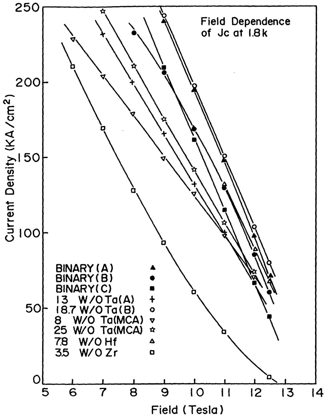
Figure 1. Critical current densities of binary and ternary alloy superconductors
