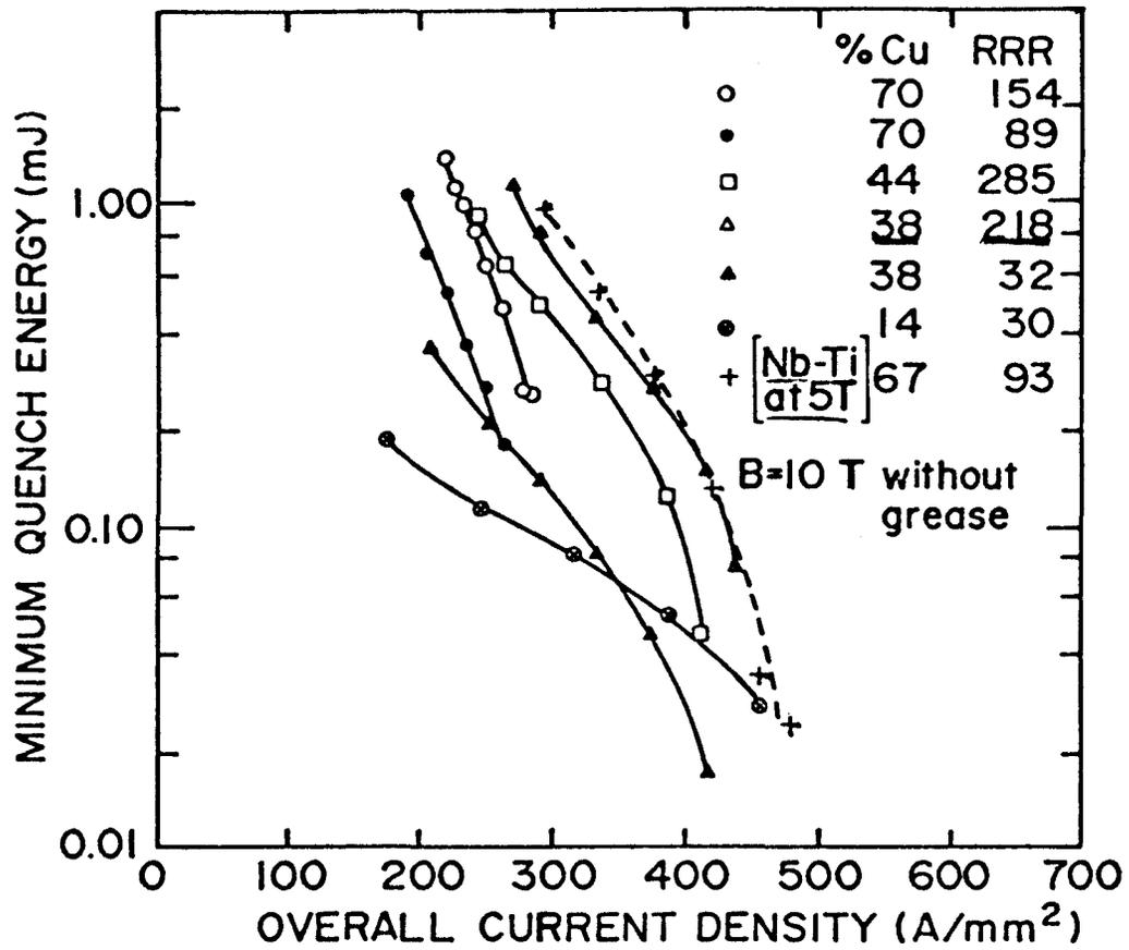
Figure 3. Minimum quench energy versus transport current density for Nb<sub>3</sub>Sn wires in liquid helium
