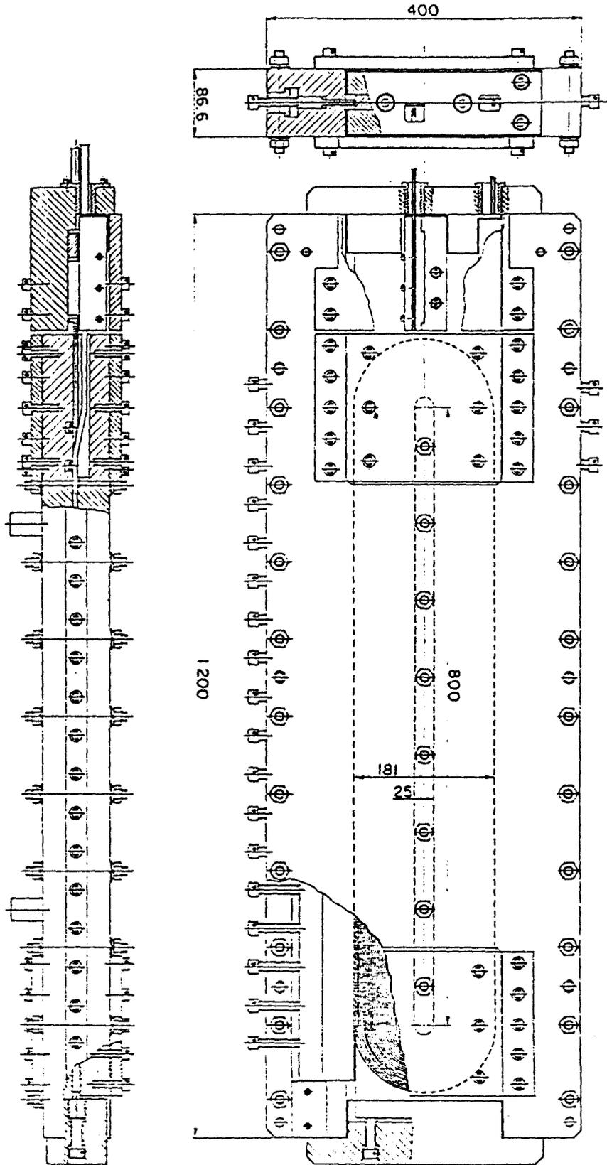
Figure 4. Structure of  $\text{Nb}_3\text{Sn}/\text{Cu}$  race-track coil magnet
