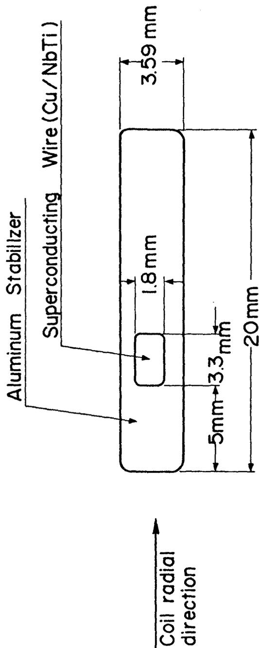
Superconducting Wire :  $50 \mu\text{m}\phi \times 1400 (2.75\text{mm}^2)$
