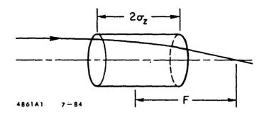
Fig. 1. The effect of the intense fields in a bunch on a particle of the opposite sign passing through the bunch.
