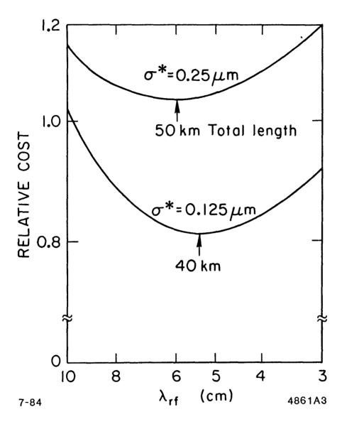
Fig. 3. Relative cost of a 2 TeV, 10<sup>33</sup> luminosity collider as a function of RF wavelength for two different final spot radii.
