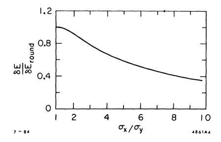
Fig. 4. Ratio of synchrotron radiation energy loss for an elliptical beam and a round beam as a function of the aspect ratio of the elliptical beam.
