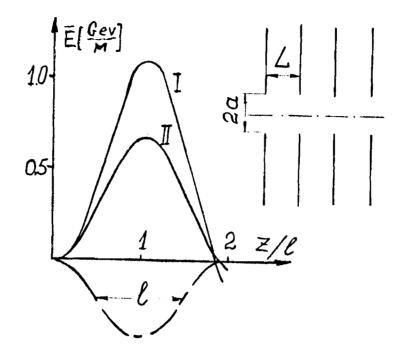
Fig. 2. Distribution of the accelerating (for electrons) field along the bunch; the number of particles  $N = 10^{13}$ , the longitudinal size of the bunch l = 0.5 cm, Q/l = 0.5, (1) L/l = 1, (II) L/l = 2.5
