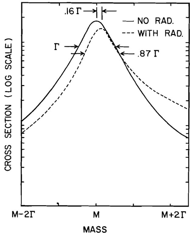
Figure 1:  $Z_0$  cross section with and without initial state radiation.
