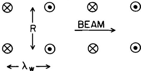
This magnet has dipole and sextupole fields but no quadrupole fields.  $R$  must be chosen large enough to make the sextupole fields small. Choose  $\lambda_w = 1\text{m}$  to put the photons generated into the X-ray region, and  $R=0.2\text{m}$
