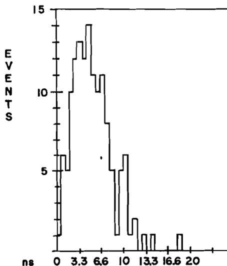
Figure 3. Timing dispersion of a single scintillator sheet.
