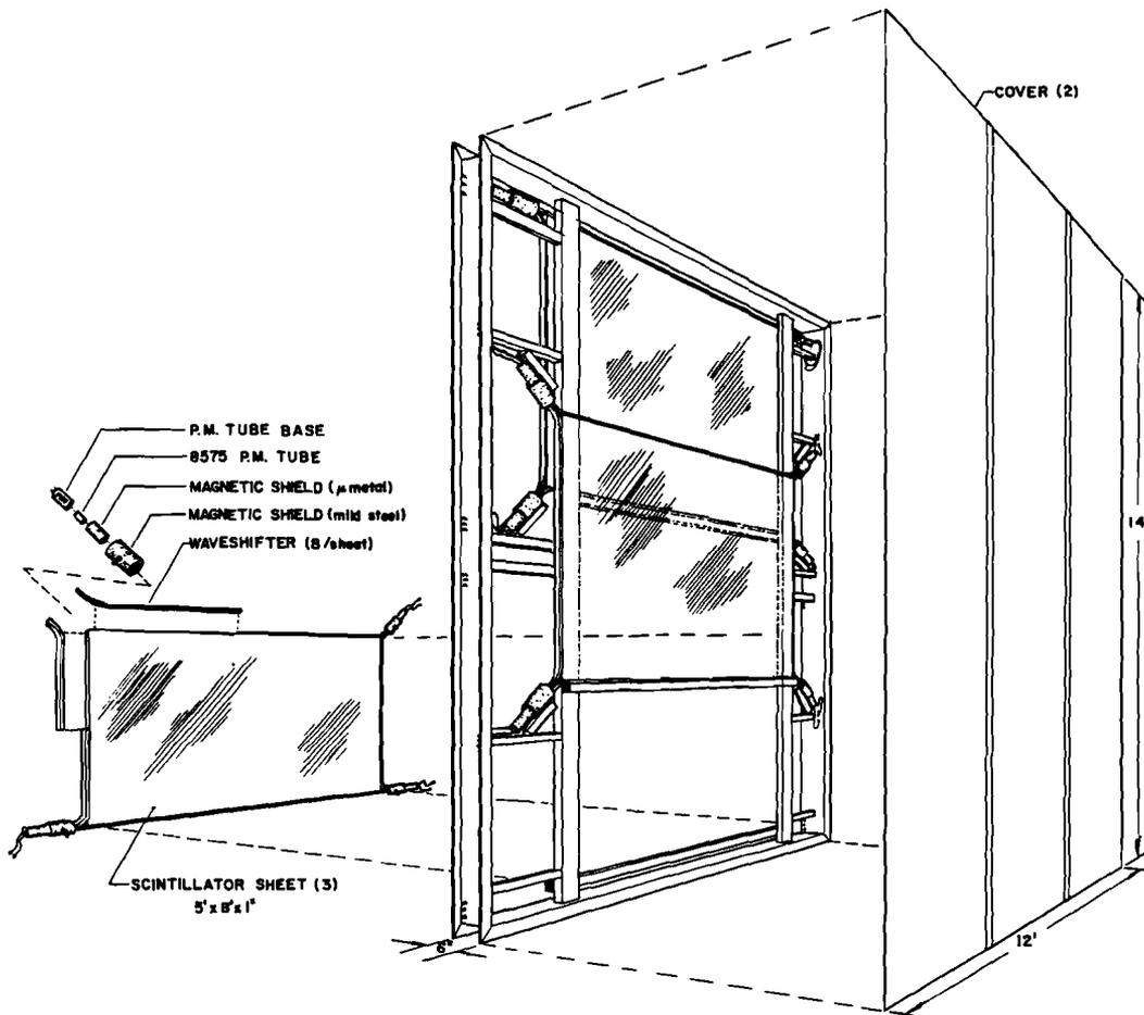
Figure 1. Structural features of a scintillator plane.
