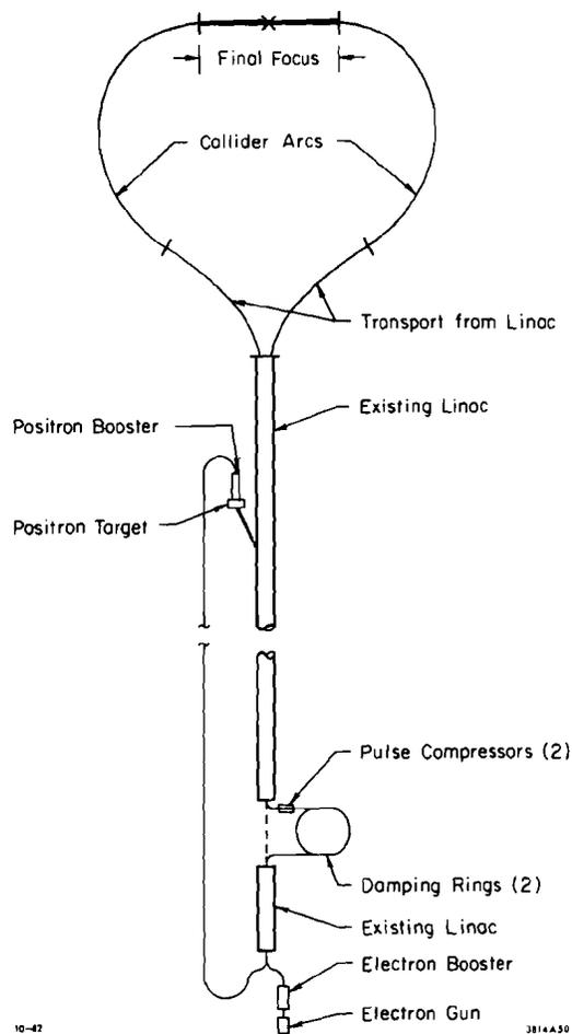
Fig. 1. Schematic layout of the SLC.
