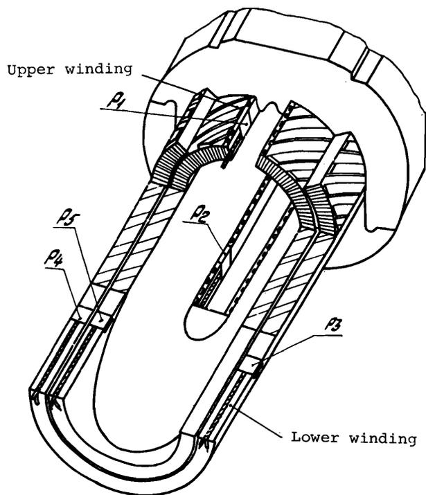
Fig. 4 Layout of the double-shell windings
