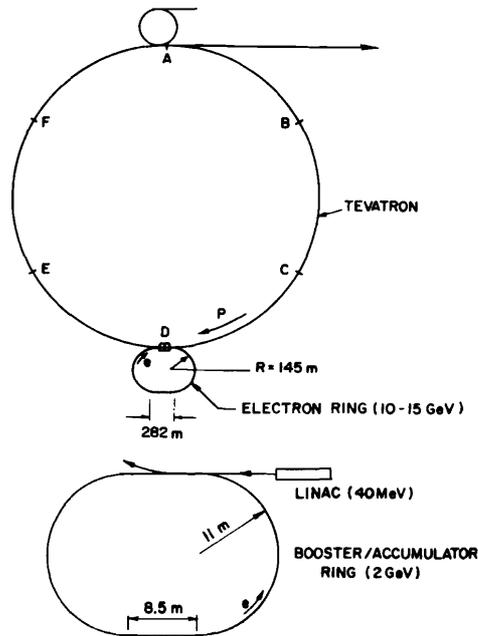
Fig. 4 Possible location of an electron ring at the Fermilab Tevatron.
