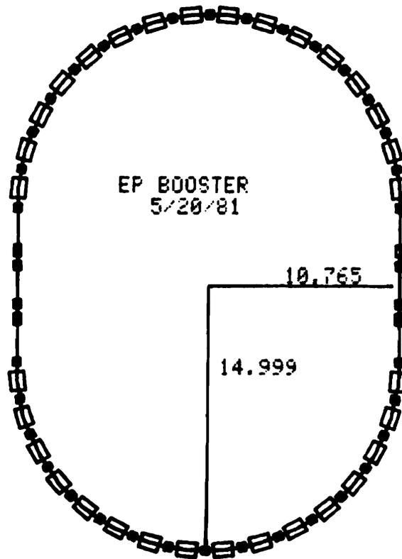
Fig. 7. The 2 GeV booster ring layout .
