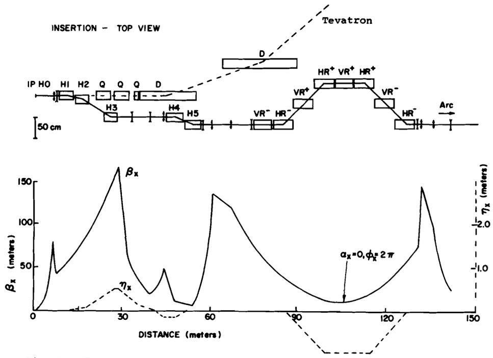
Fig. 6a The interaction straight section at the Tevatron. The dashed line is the proton orbit.
