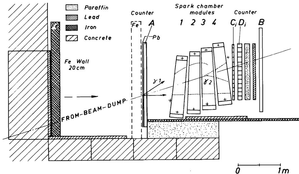
Fig. 1: Experimental arrangement at SIN.<sup>23,33</sup>) A complete  $2\gamma$ -event (class AB) is drawn in. - The  $3 \times 2\ \text{m}^2$  large iron wall "Fe" was in front of the decay region ( $d = 2\text{m}$ ), through part of the effect runs, and at its end (dashed) for the "Null-Test" (see text).
