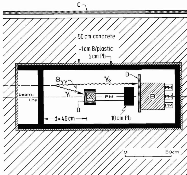
Fig. 5: Set-up for the reactor experiment at Jülich. - A and B are the essential (NaI)-counters, C and D plastic veto-counters.
