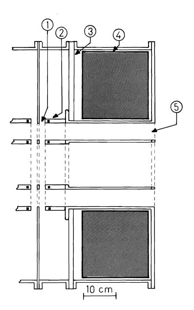
Figure 1. Pulselac C Acceleration Module. 1) Magnetically insulated acceleration gap. 2) Coaxial drift tube structure with magnetic coils. 3) Vacuum insulator. 4) Ferrite core (250 kV, 50 nsec). 5) Annular drift region.
