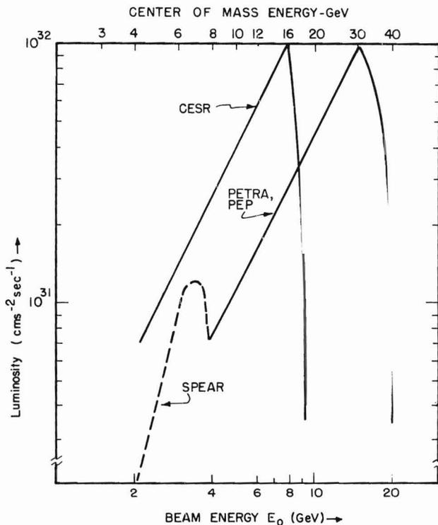
Fig. 5 A comparison of the design luminosity of CESR, PEP, PETRA. The performance of SPEAR is also shown.
