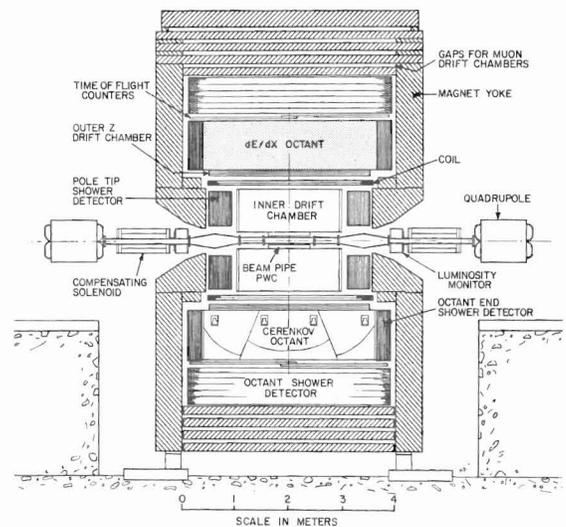
Fig. 9 The CLEO magnetic detector as viewed perpendicular to the beam line.
