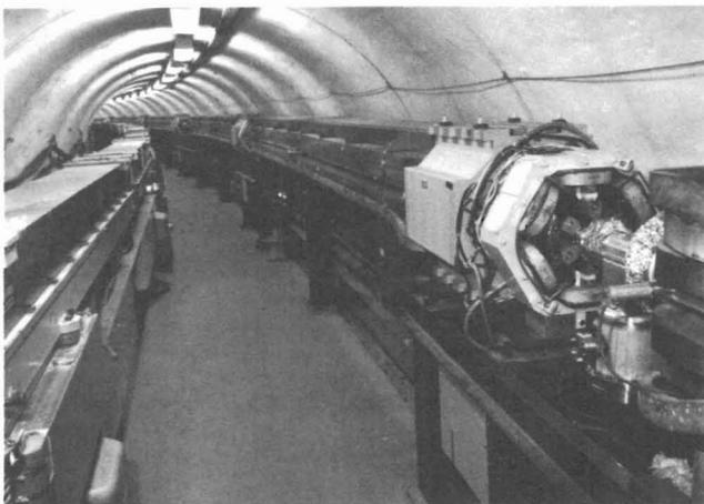
Fig. 2 Tunnel interior with the CESR guidefield magnets shown on the right and the synchrotron magnet ring on the left.
