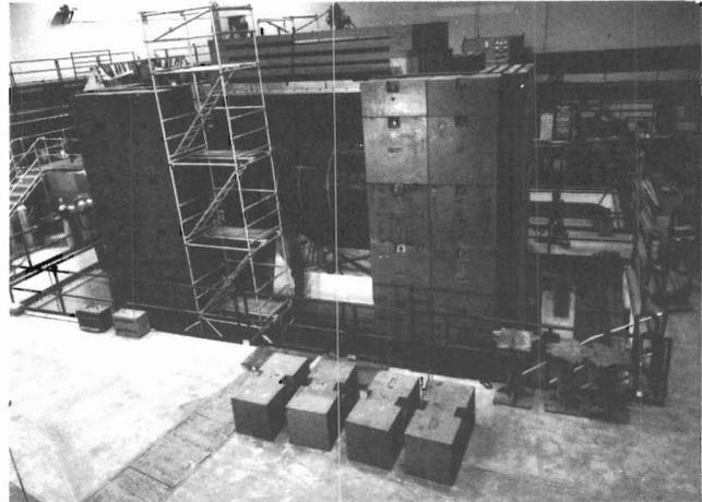
Fig. 13 Exterior view of CLEO. This view shows the solenoid in place together with one of the octants below. The outer muon shields have been parted to provide access.
