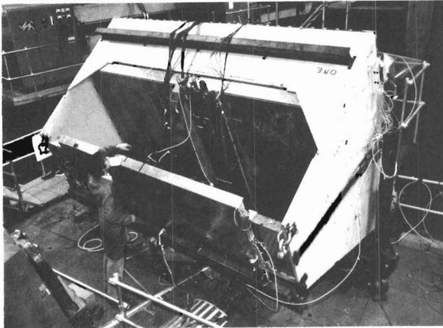
Fig. 11 A view of a partially assembled octant of the CLEO detector.
