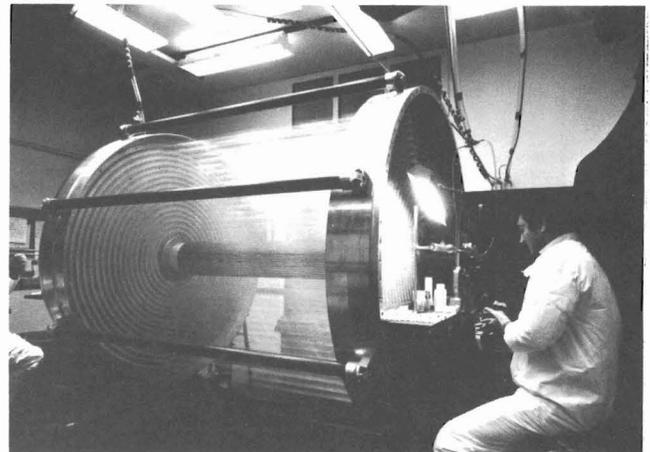
Fig. 10 View of the central drift chamber of CLEO during construction. More than 5,000 cells are provided, arranged in 17 layers.
