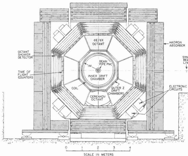
Fig. 8 The CLEO magnetic detector as viewed along the beam line.
