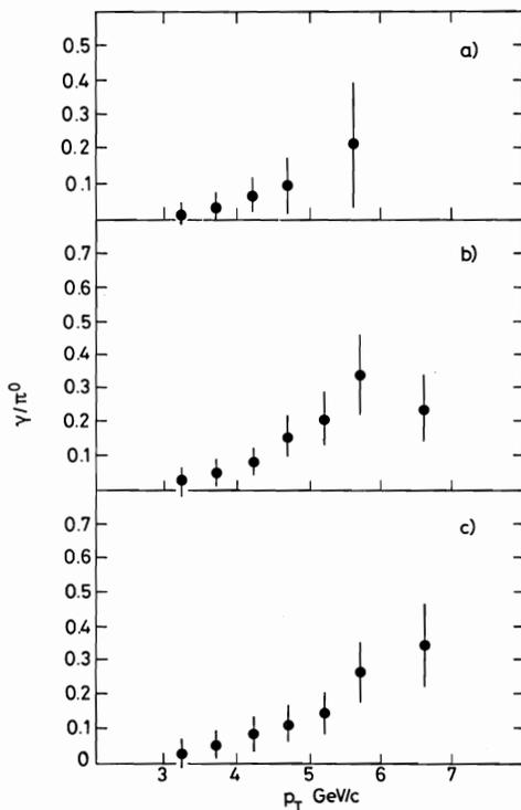
Figure 4 : Final results for the  $\gamma/\pi^0$  ratio from configuration A. The contribution of  $\pi^0$  and  $\eta$  decays has been subtracted and a correction applied for reconstruction efficiency. The errors include all systematics: (a) for  $\sqrt{s} = 31$ , (b) for  $\sqrt{s} = 53$ , and (c) for  $\sqrt{s} = 62$  GeV.
