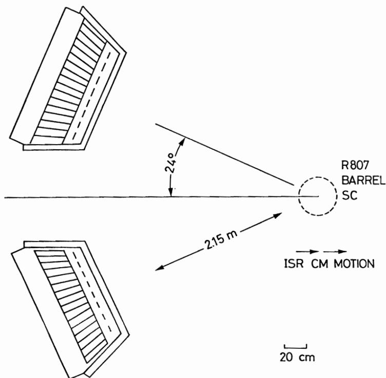
Figure 2 : Arrangement of the calorimeter modules for the study of single photon production at large  $p_T$  (configuration B).
