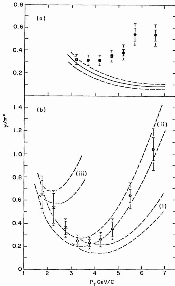
Figure 3a : Observed ratio of  $\gamma$  to  $\pi^0$  for data from all energies for configuration A. The inner error bars indicate statistical errors. The outer bars indicate possible systematic effects due to calorimeter non-linearity. The smooth line indicates the Monte Carlo prediction for the ratio assuming no direct  $\gamma$  production. The dashed lines indicate the one standard deviation systematic errors on the Monte Carlo calculation.
