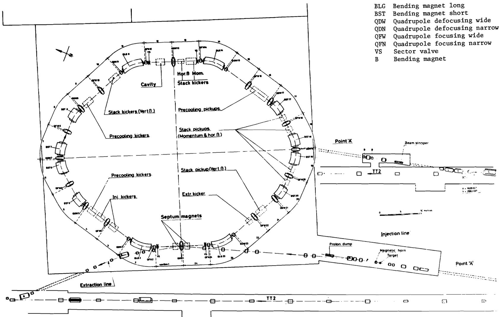
Fig. 5. General layout of the antiproton accumulator
