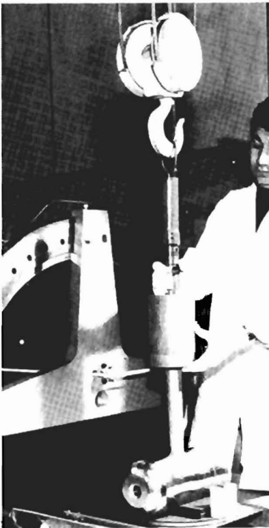
◀ Fig. 11. Drift tube being loaded on special cart.
