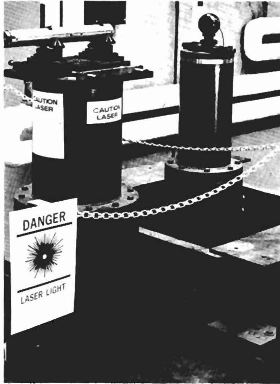
Fig. 3. Primary alignment monument station at Station 0.00.
