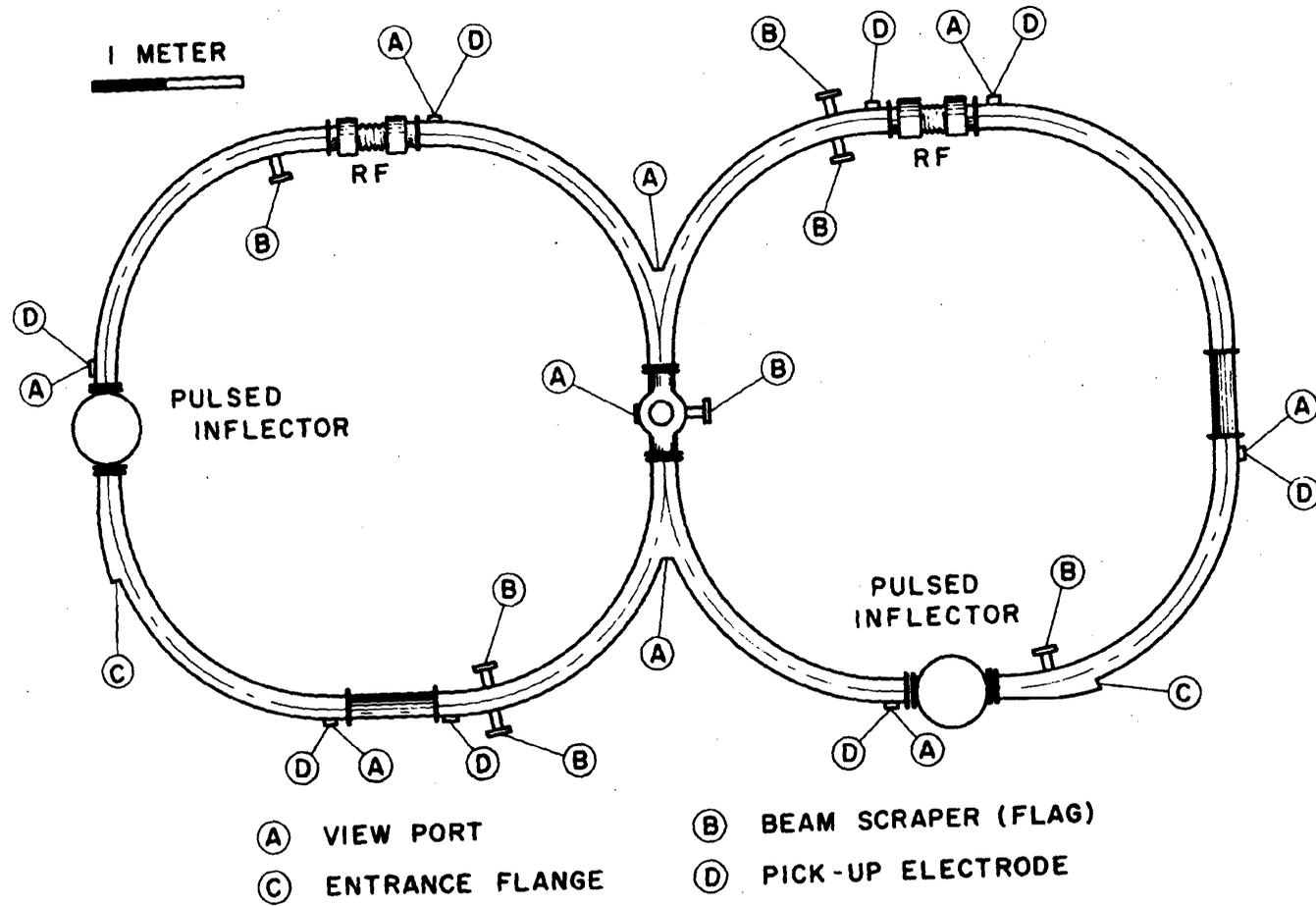
Fig. 1 - Vacuum chamber for the storage rings
