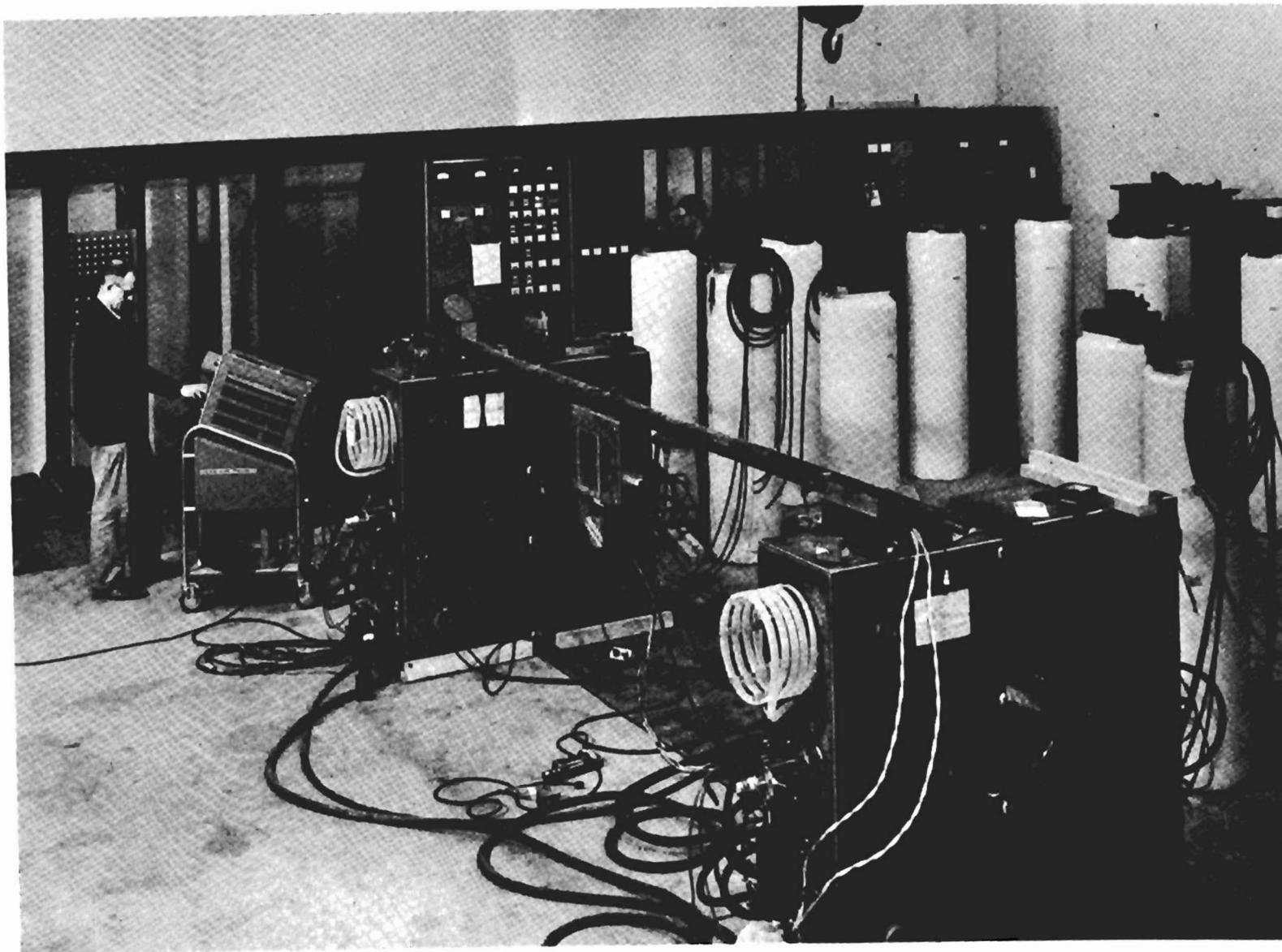
Fig. 2 - Split rf cavities for the storage rings
