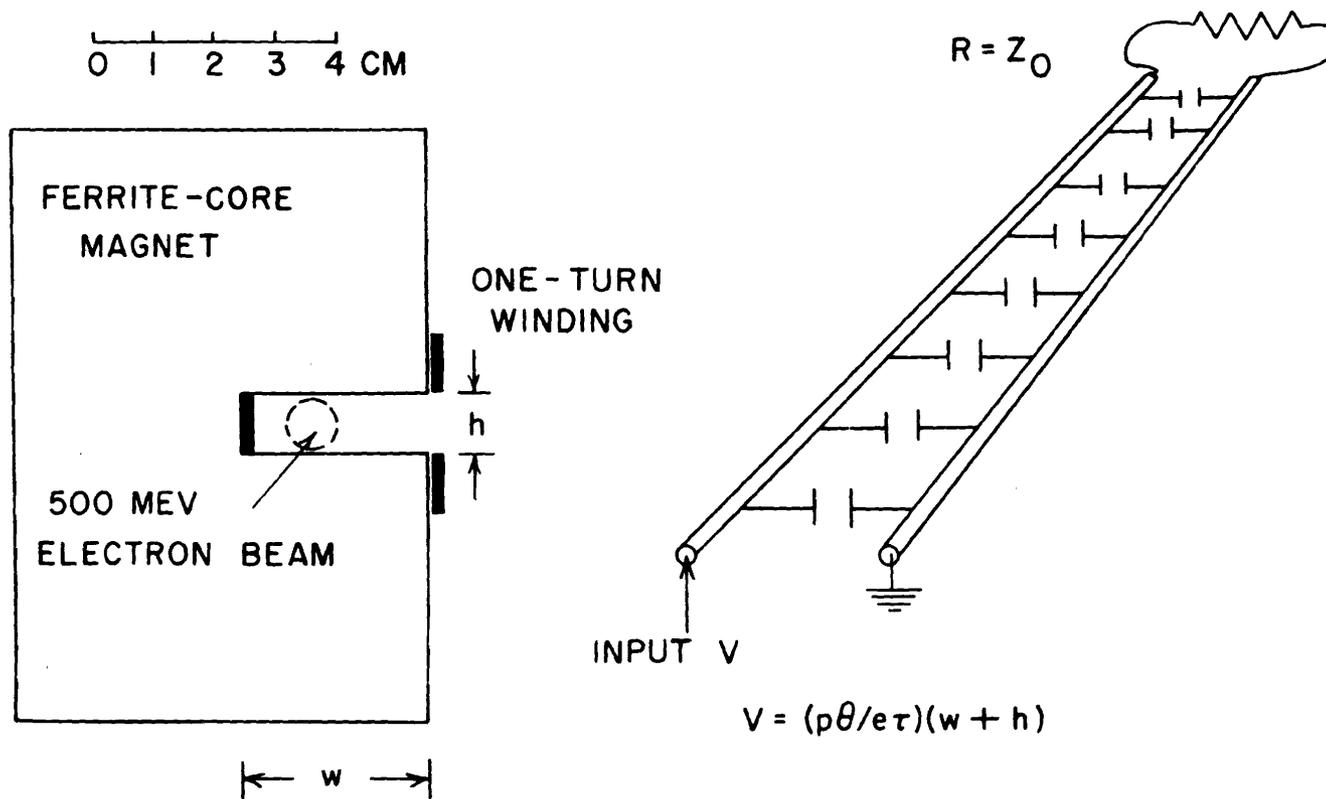
Fig. 7 - Schematic of the delay-line inflector
