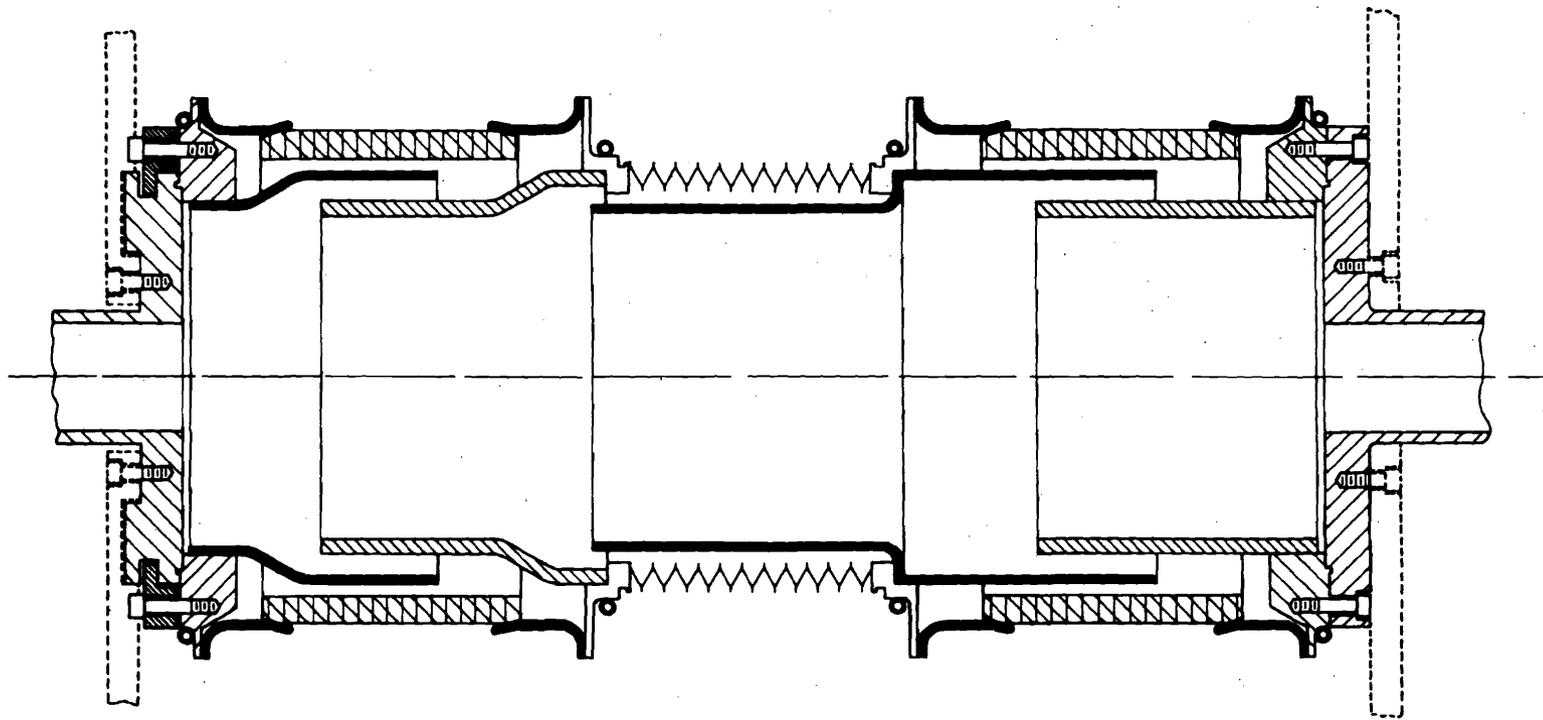
Fig. 4 - RCA "ramseals" for high-vacuum rf gaps
