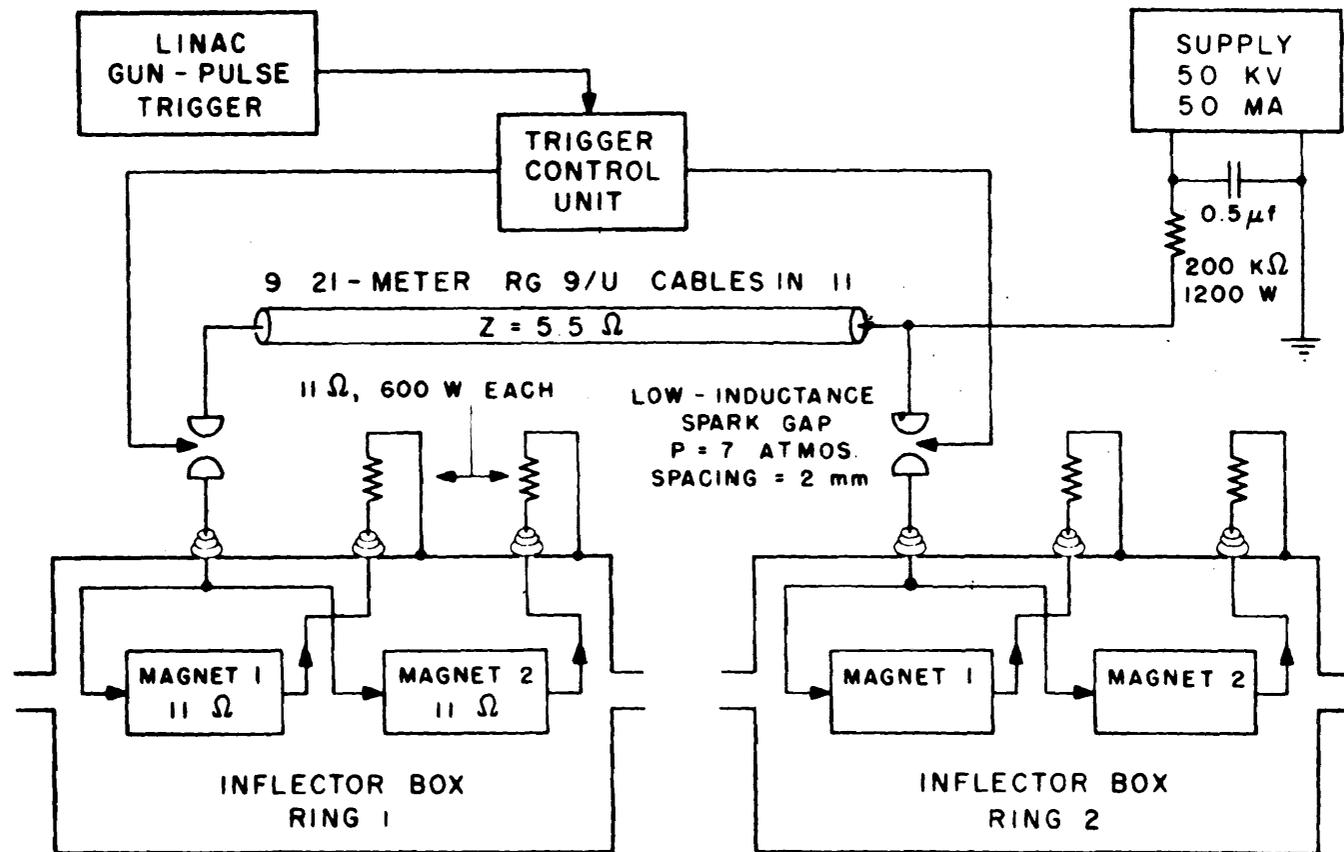
Fig. 8 - Circuit for pulsing the delay-line inflector
