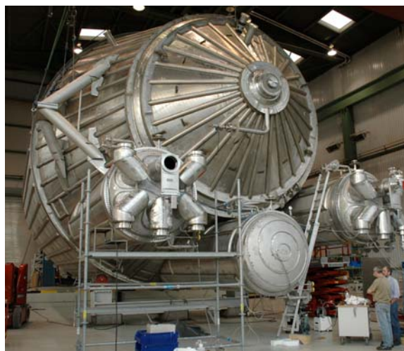
Figure 5. The very large - the KATRIN main spectrometer vessel nears completion.
