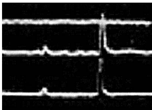
Figure 8. A typical scope trace of a delayed-coincidence signal.
