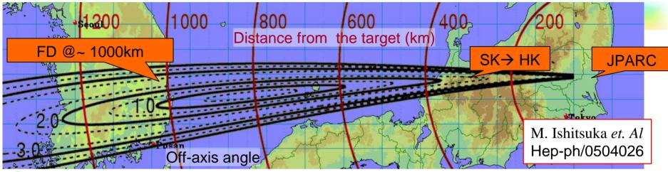
Far detector identical with (SK)/HK @ 2<sup>nd</sup> Oscillation Maximum point.
