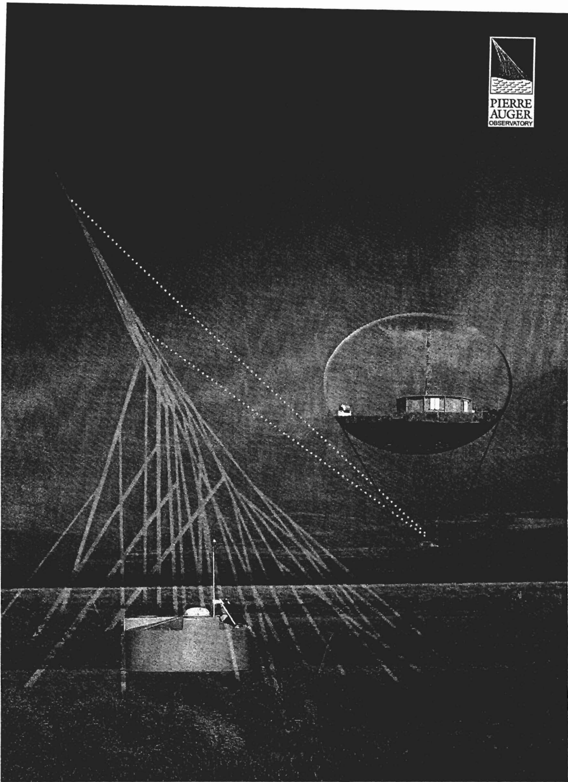
Illustration of the detector systems used in the Pierre Auger Project. Self-contained particle detectors are spaced on a 1.5 km grid over the surface. The air showers are also observed on dark nights using air fluorescence telescopes (inset).
