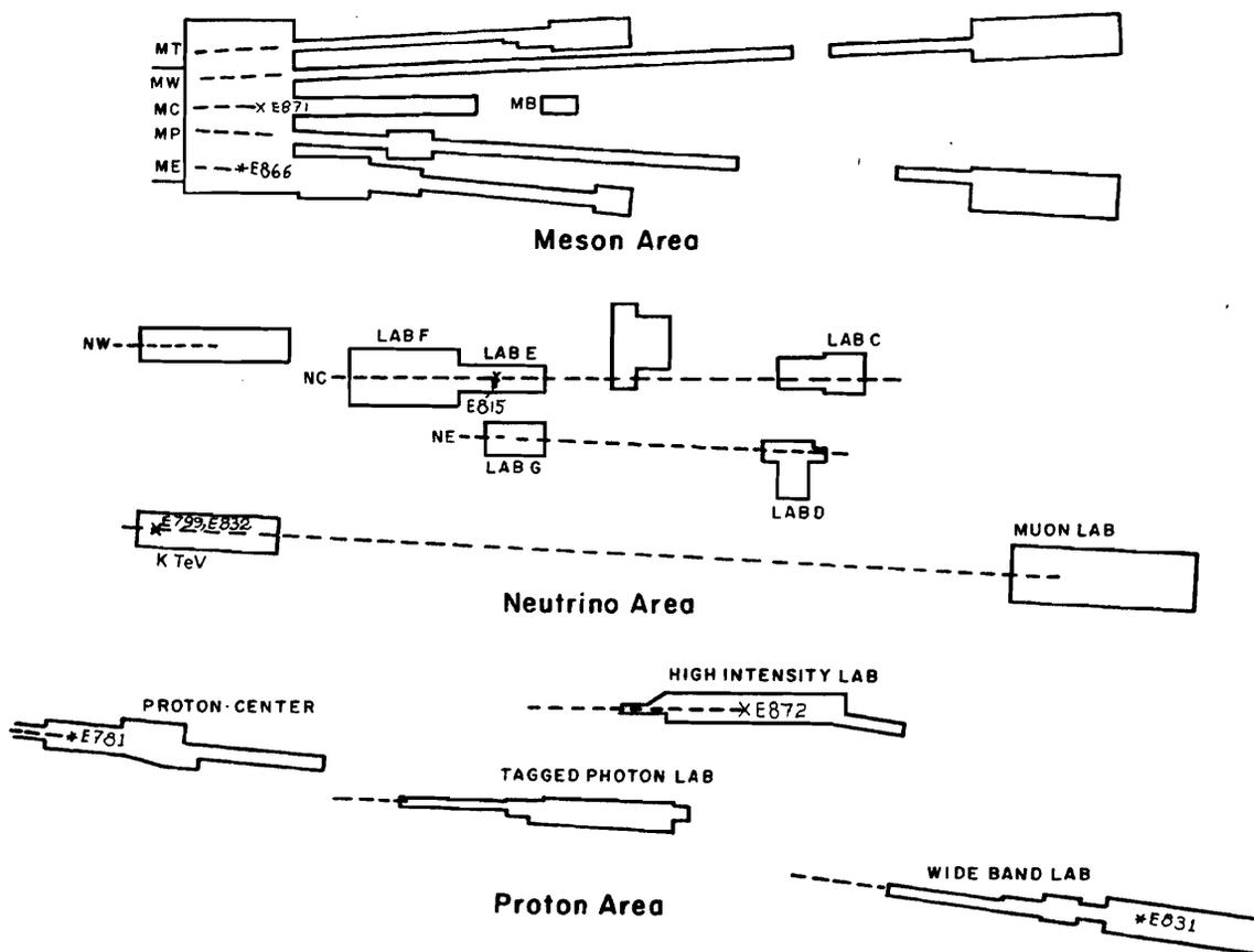
Figure 9. Schematic of the Fixed Target experimental areas with locations of major experiments currently approved for the next Fixed Target run. Not shown are experiments E-803 and E-875, which will use a neutrino beam from the Main Injector. The drawings are not to scale.
