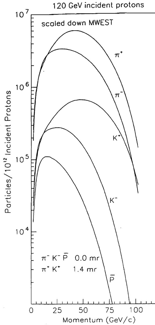
Figure 18. Main Injector: Fluxes in the MW beamline.
