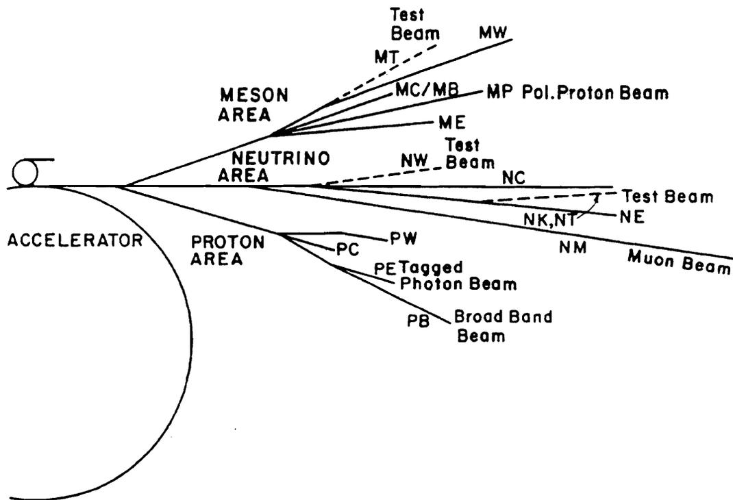
Figure 8. Layout of Fermilab Fixed Target beams. Properties of individual beams are given in Table 2.
