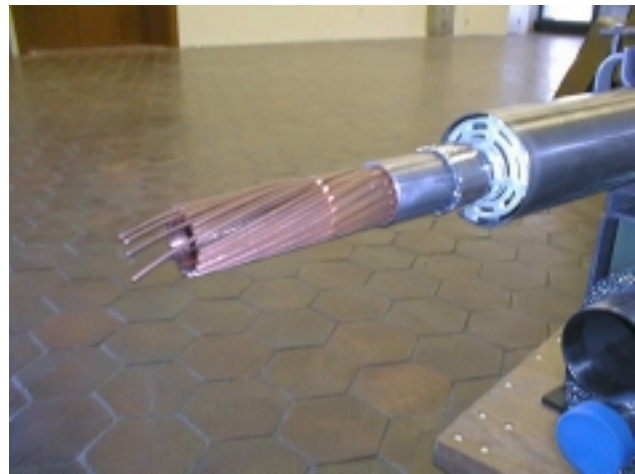
Figure 11 – Photograph of transmission line conductor at end of 2m model magnet. From left to right: NbTi superconducting strand, helically-slit copper stabilizer, Invar cryogenic pipe, vacuum superinsulation, G-10 support “spider”, 304 Stainless Steel vacuum jacket, and body of transmission line magnet.
