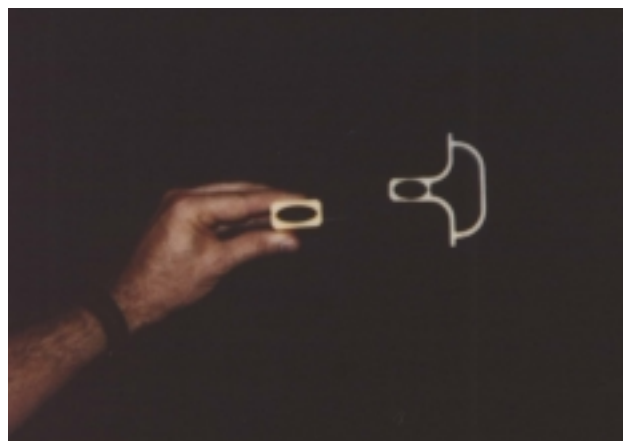
Fig. 23 – Photograph of the aluminum shelled split-tube BPM and an aluminum beam pipe test section.
