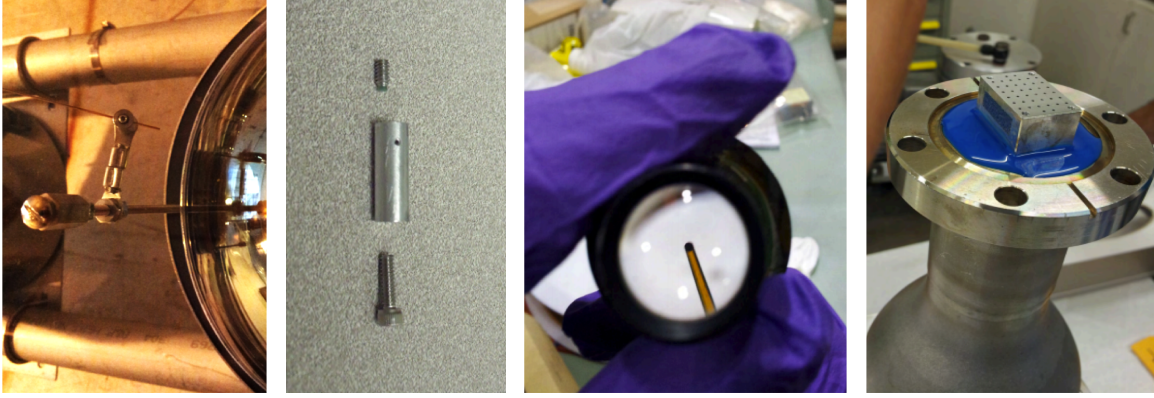
Figure 2.2.7: Left to right: the mounting stand-off which holds the fiber at each PMT; the stainless steel standoff with its nylon-tipped set-screw; magnification of the prepared fiber end, which points towards the photocathode; connector block being set in the custom feedthrough. From [3].
