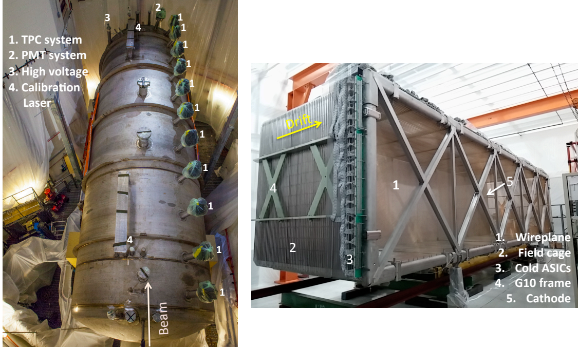
Figure 2.1.2: Left: Top view of the MicroBooNE cryostat in situ in the beamline, showing the locations of cable feedthroughs for each active system. Right: Side view of the MicroBooNE TPC during construction.
