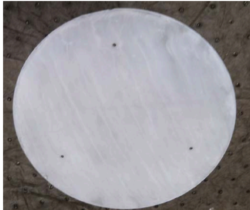
Figure 2.4.2: Left: Cartoon showing the TPB plate emission in transmission mode. Purple lines represent incident VUV photons, blue lines are emitted visible photons, and grey lines represent lost light. Right: photograph of a coated MicroBooNE plate.
