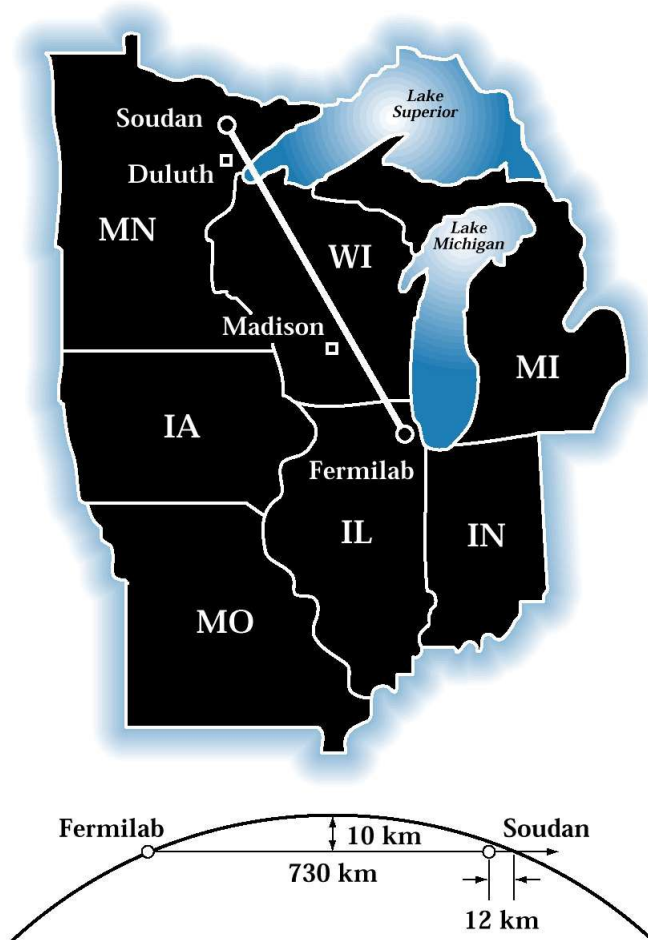
Figure 3.1: The MINOS neutrino beamline. The \nu_\mu/\bar{\nu}_\mu beam is produced in the NuMI facility at Fermilab. It passes through the ND at Fermilab and the FD in the Soudan mine in northern Minnesota. The baseline is 735 km. The figure is taken from Reference [73].
