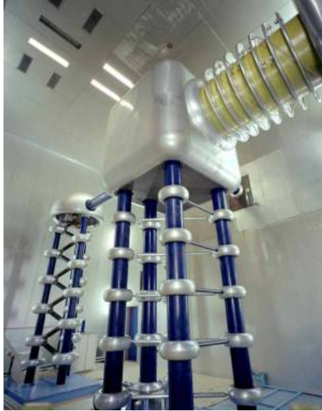
Figure 5.2: The pre-accelerator at Fermilab, which takes H^- ions and accelerates them to an energy of 750 keV.
