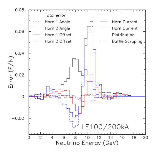
Figure 5.27: The summary of far over near ratio uncertainties due to proton beam and focusing uncertainties for the LE100/200kA beam. The uncertainties were calculated using distortion functions that were found as described in Sections 5.2.1-5.2.4 and an estimate of the size of each uncertainty based upon NuMI beam-line instrumentation data (Table 5.1). The total uncertainty is given as a sum of all uncertainties in quadrature.
