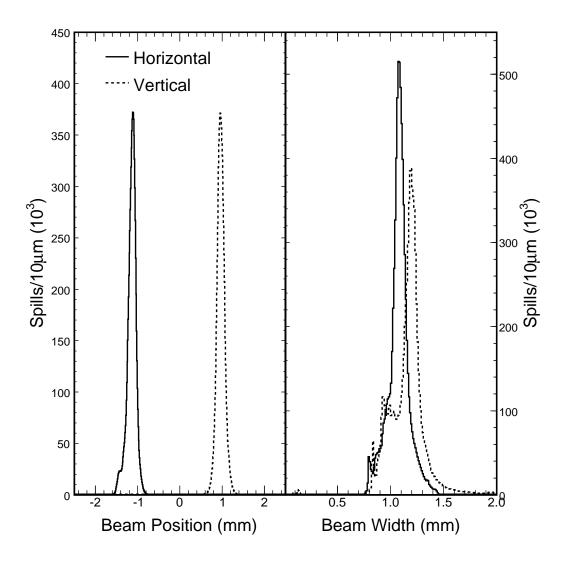
Figure 2.7: Primary proton beam position and width at the target. Data accumulated with first NuMI target corresponding to  $1.57 \times 10^{20}$  POT. During the running the beam was centered on the target (Figure 2.6) and the beam width was relatively small compared to the  $6.4 \times 18 \text{ mm}^2$  profile of the target.
