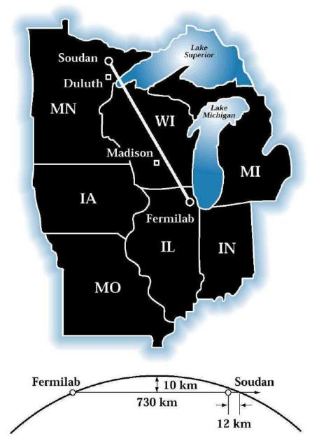
Figure 2.1: A geographical layout of MINOS detectors. The source of neutrinos for MINOS experiment is Fermilab's NuMI beam-line. The beam is steered toward the two MINOS detectors. The Near Detector (ND) is located close to the source of neutrinos on Fermilab site, while the Far Detector (FD) is 735 km away in the Soudan mine, Minnesota. Figure taken from [32].
