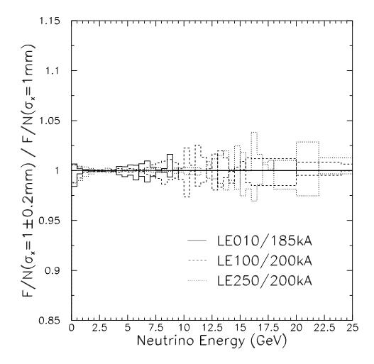
Figure E.1: The curves represent the changes in far over near ratio for  $\pm 20\%$  excursions in the proton beam width  $\sigma_x$ . Excursions by  $\pm 10\%$  produce approximately half as large of an effect on the F/N ratio.
