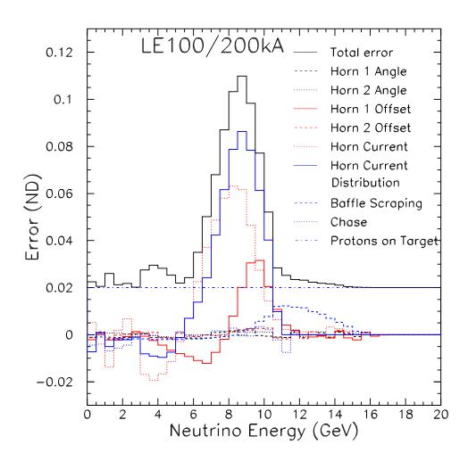
Figure 5.24: The summary of neutrino energy spectrum uncertainties at the ND due to proton beam and focusing uncertainties for the LE100/200kA beam. The uncertainties were calculated using distortion functions that were found as described in Sections 5.2.1-5.2.4 and an estimate of the size of each uncertainty based upon NuMI beam-line instrumentation data (Table 5.1). The total uncertainty is given as a sum of all uncertainties in quadrature.
