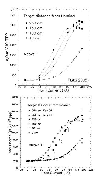
Figure C.12: Muon rates in Alcove 1 as a function of the horn current for several target positions. (top) Prediction from the GNuMI beam MC with Fluka 2005 input hadrons off the target. The lines are polynomial fits to the MC points to guide the eye. (bottom) NuMI data taken in 2005-2006 [108]. A background of  $35 \pm 7 \text{ pC}/10^{12} \text{ ppp}$ , due to particles produced in the beam absorber, expected to be independent of horn current, has not been subtracted from these data.
