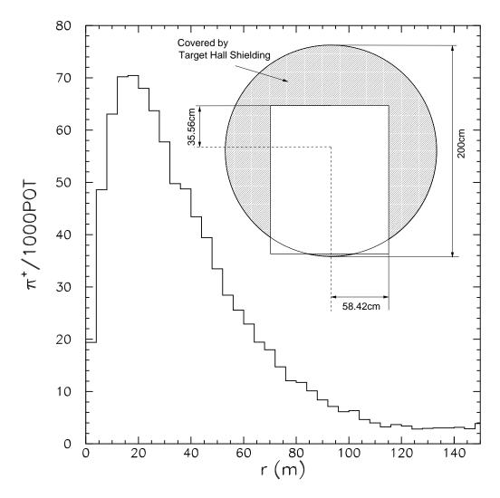
Figure 3.18: The expected radial distribution of pions at the location of the upstream window ( $\sim$ 45 m away from target) if no shielding was present in the target hall. The inset shows the beam view of the entrance to the decay pipe from the target hall. The shaded region indicates is the aperture of the shielding in the Target Hall. The decay pipe is centered on the beam axis.
