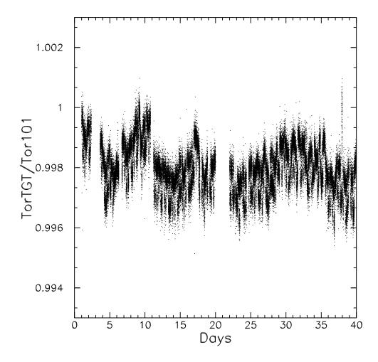
Figure 5.4: Plot of the ratio of two NuMI toroids, TorTGT and Tor101, plotted over a long period of time (Data from August 10th - September 20th 2005). The drift in this ratio by  $\pm 0.2\%$  is similar to the magnitude of the drift observed in the toroids' pedestal values.
