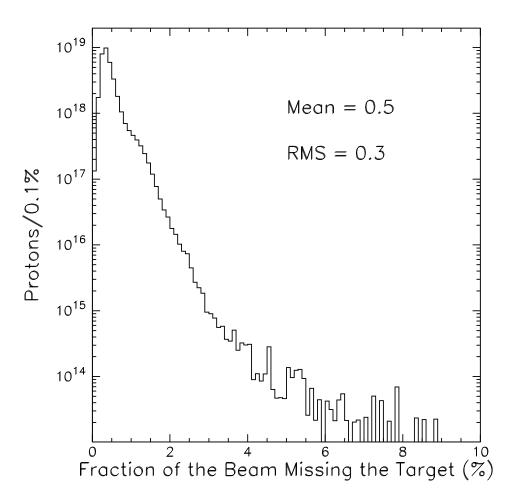
Figure 5.6: The proton beam has a spot size of  $\sigma_x \times \sigma_y \approx 1.1 \times 1.2 \text{ mm}^2$ which is comparable to the target width of 6.4 mm (see Figure 2.6). A certain number of protons misses the target depending on the beam position and width. Shown is the fraction of the beam missing the target over a period of few months of normal running.
