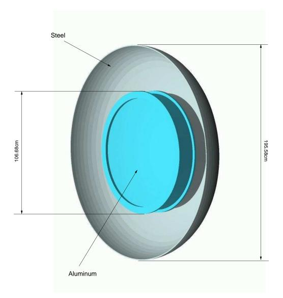
Figure 3.19: The 3d view of the upstream Decay Pipe Window. The window keeps the vacuum seal in the decay pipe. The inner part of the window, which mostly overlaps with the aperture of the Target Hall (see Figure 3.18), is made out of Aluminum in order to reduce the reinteraction of particles as they pass through the window.
