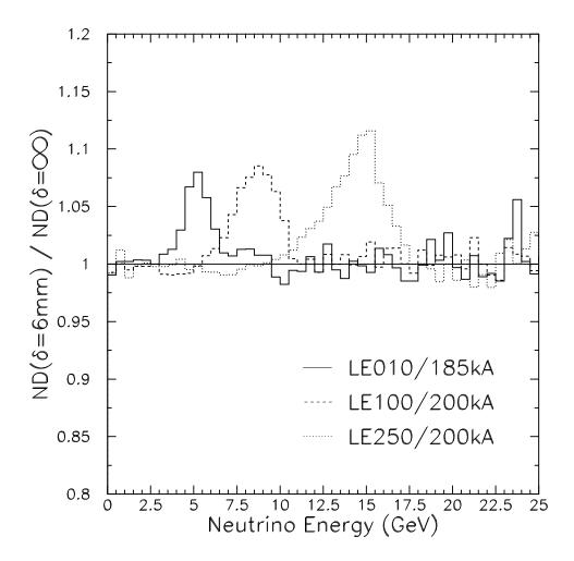
Figure 5.22: The ratio of neutrino fluxes at the Near Detector where different distributions of horn current inside the inner conductor were used to calculate the fluxes. The current distribution affects the distribution of the magnetic field and consequently what is the highest momentum of the particles being captured by a horn. Shown is the difference between the skin depth  $\delta = 6$  mm and  $\delta = \infty$ .
