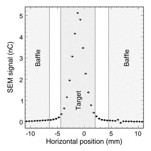
Figure 2.6: Distribution of protons in horizontal plane for a spill centered at x=1.1 mm with width  $\sigma_x = 1.2$  mm. Indicated is the location of the target and the baffle during the first run period as determined in [41].
