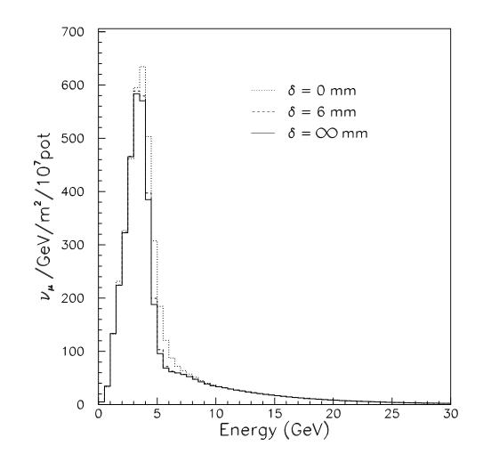
Figure 5.21: The neutrino flux at Near Detector for two extremal distributions of current in horn inner conductor. Three current distributions correspond to different skin depths  $\delta = 0, 6$  mm, and  $\delta = \infty$ .
