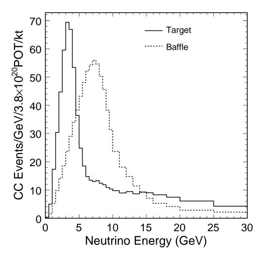
Figure 5.8: The collimating baffle located upstream of target is made of graphite and can act as another target. As per variable energy beam concept (§2.1.2) this produces higher energy neutrino spectrum. Shown is the neutrino spectra at the far detector corresponding to beam centered on target and beam hitting directly on baffle.
