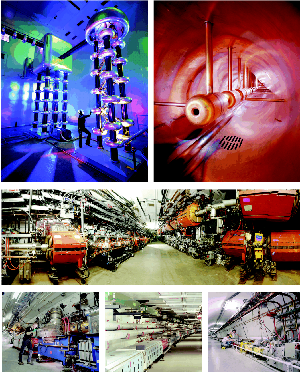
Figure 5. Photographs of components of the Fermilab accelerator complex: (top left) the Cockcroft-Walton preaccelerator, (top right) the interior of one of the Linac drift tubes, (center), the Debnuncher and Accumulator, (bottom left), the Booster, (bottom center), the Main Injector, and (bottom right) the Tevatron.
