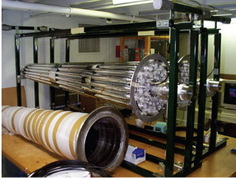
Figure 2.28. The Cherenkov Luminosity Detector is made up of two of these modules, one on each side of the detector.
