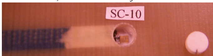
Fig. 5.13: Temperature sensor under the NEMA layer with the groove for the wires, and a hole for the temperature sensor; a cap of RTV-impregnated fiberglass protects the sensor.
