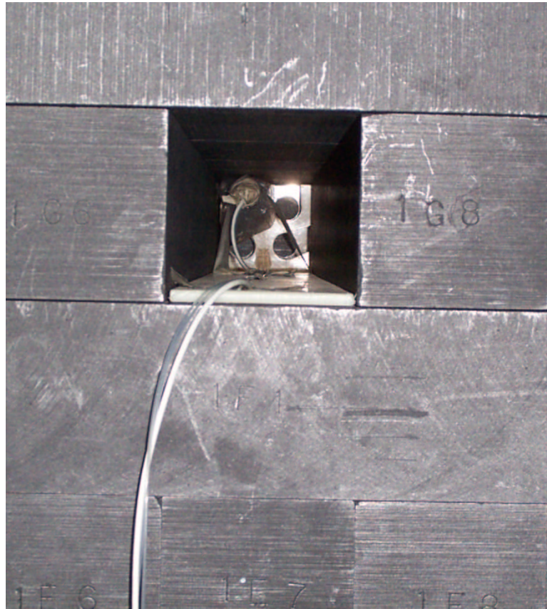
Figure 6: Thermal neutron calibration of the TE ionization chambers at the Oregon State University Research Reactor. Here a detector has been placed on a plastic holder and inserted into the thermal column of the reactor.
