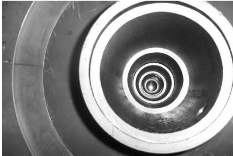
Figure 27: Photograph of the 20-cm diameter collimator inserted into the Fermilab Neutron Therapy Facility.
