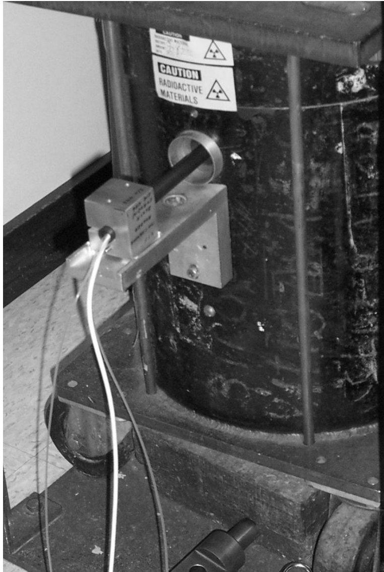
Figure 5: ^{137}\text{Cs} calibration source located in the Fermilab Neutron Therapy Facility treatment room. The source was used for checking the proper operation of the ionization chambers before use.
