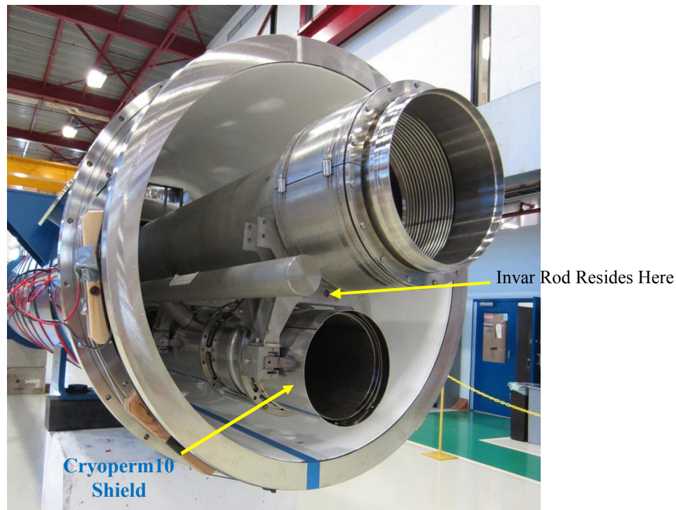
Figure 1. Partially Assembled Cryomodule
