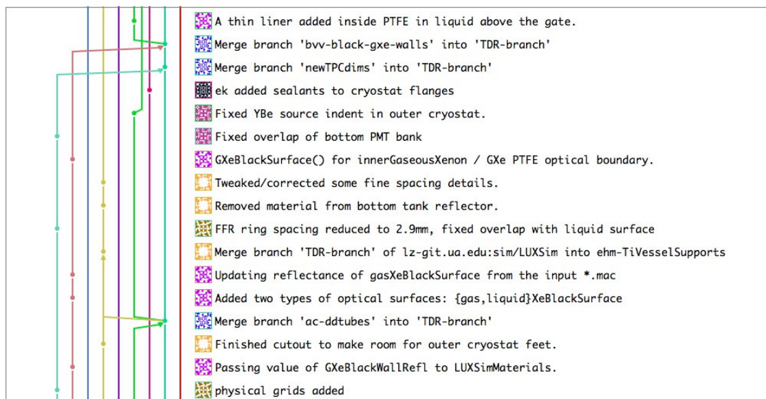
Figure 11.5.1: Parallel development workflow in GitLab: several contributors were updating the LZSim detector geometry simultaneously. Each vertical line corresponds to a different development branch. After extensive testing, every update was eventually merged to the master branch.
