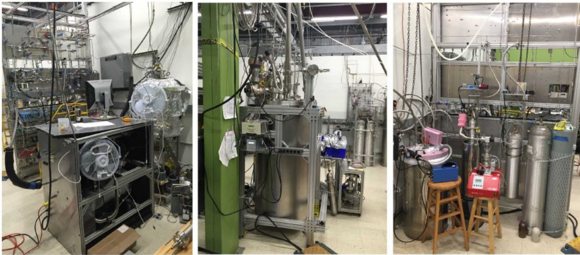
Figure 6.3.1: The three panels show the Kr removal development platform. Left: the gas control manifold, pumps, and charcoal column. Center: LN thermosyphon cooled condenser for xenon recovery. Right: krypton traps and xenon feed and storage located on the back side of the manifold.
