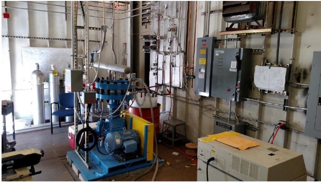
Figure 6.4.3: Fluotron 100 slpm all-metal single-stage diaphragm compressor operating as part of SLAC System Test.
