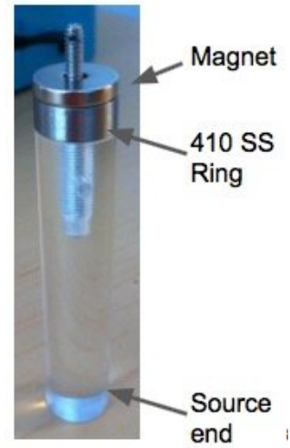
Figure 7.2.4: Prototype dummy source capsule showing 410SS ring with magnetic recovery system attached.
