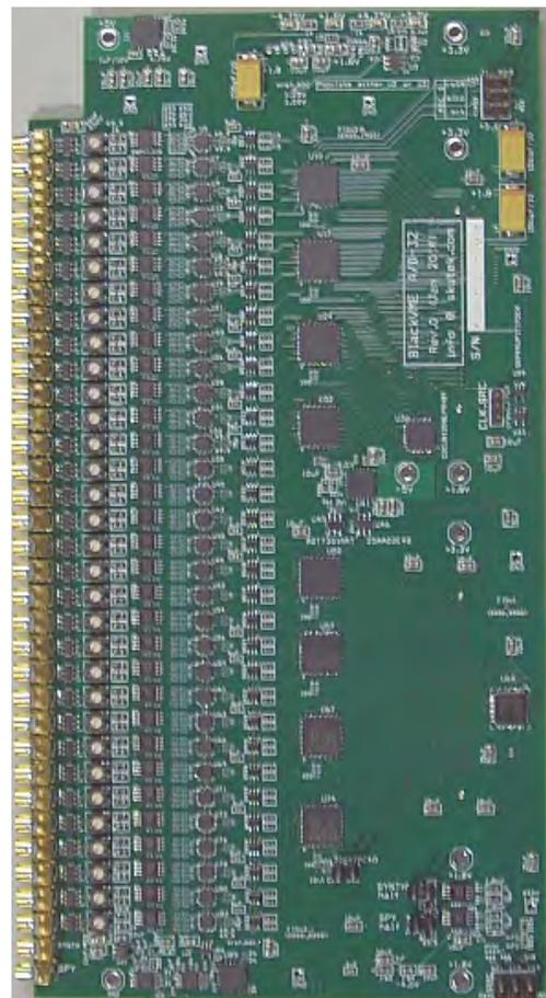
**Figure 11.4.2. Prototype ADC daughter card with 32 channels.**
