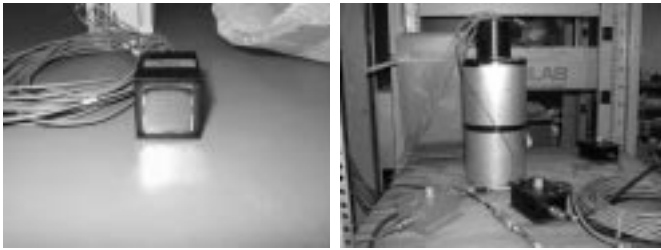
Figure 5.14: Left: The Hamamatsu R-5900 MAPMT has a 1 squared inch cross-section; Right: The test stand at the Rockefeller Lab.
