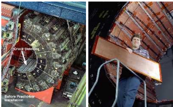
Figure 5.2: Photographs of one arch of twelve calorimetry wedges, pulled away from the beamline. The Run I preshower and crack detectors are seen lining the inner surface of the arch in the right photograph.
