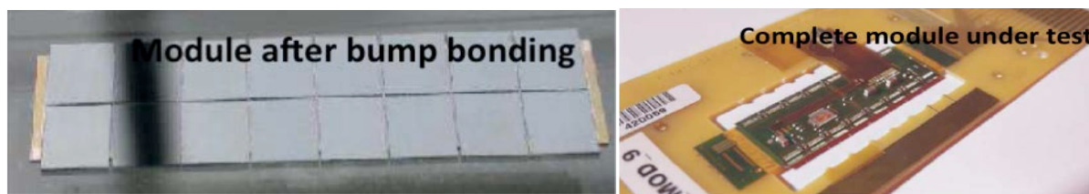
Fig. 1: Diamond sensor bump-bonded to 16 FE-I3 chips (left) and the completed ATLAS diamond pixel module under test (right).
