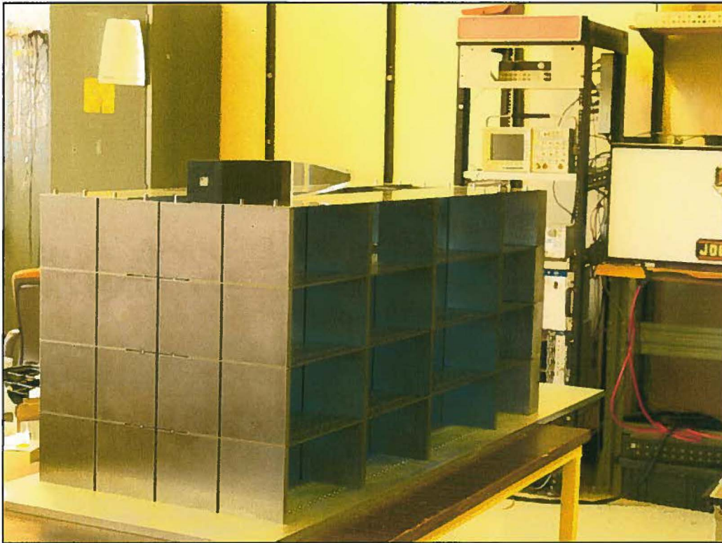
Figure 1: HAD section for STAR forward upgrade. At the top we placed one of the tungsten powder /Sc fiber EM supermodules which was tested previously at FNAL T-1018.
