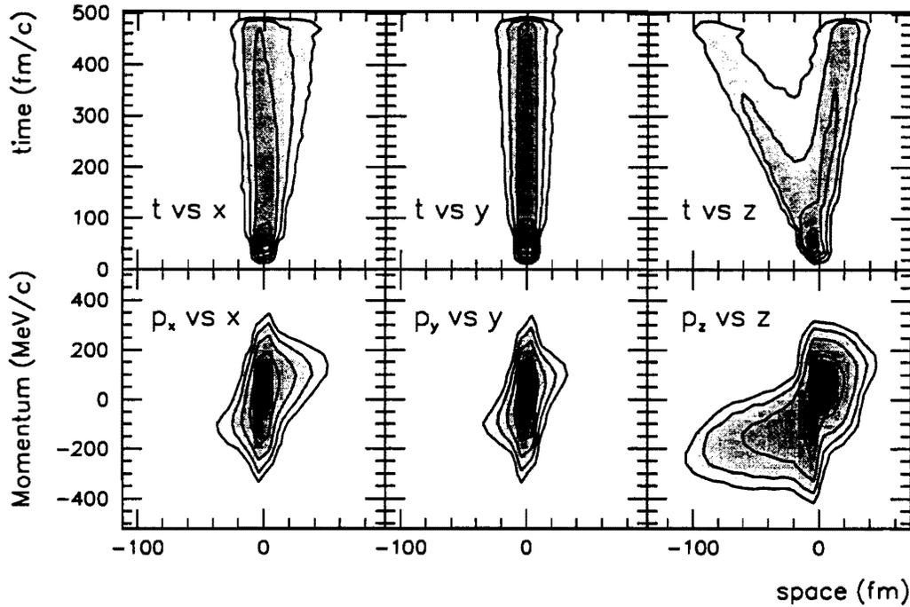
Fig. 9 Correlation between coordinates of emission points, emission times and asymptotic momenta of protons predicted by the quantum molecular dynamics model (QMD).
