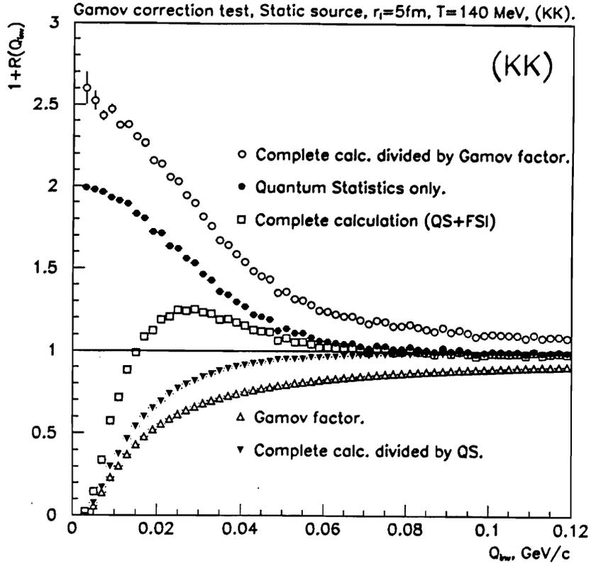
Fig. 12 Simple correction using Gamov factor cannot account for two-particle Coulomb interaction and leads to extraction of wrong parameters of fits of correlation functions (here for two kaons).
