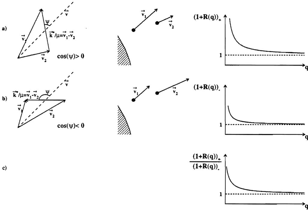
*Fig. 5 Sensitivity of the correlation function to the sign of the time difference of particle emission can be simply interpreted in the frame of the classical trajectory approach.*
