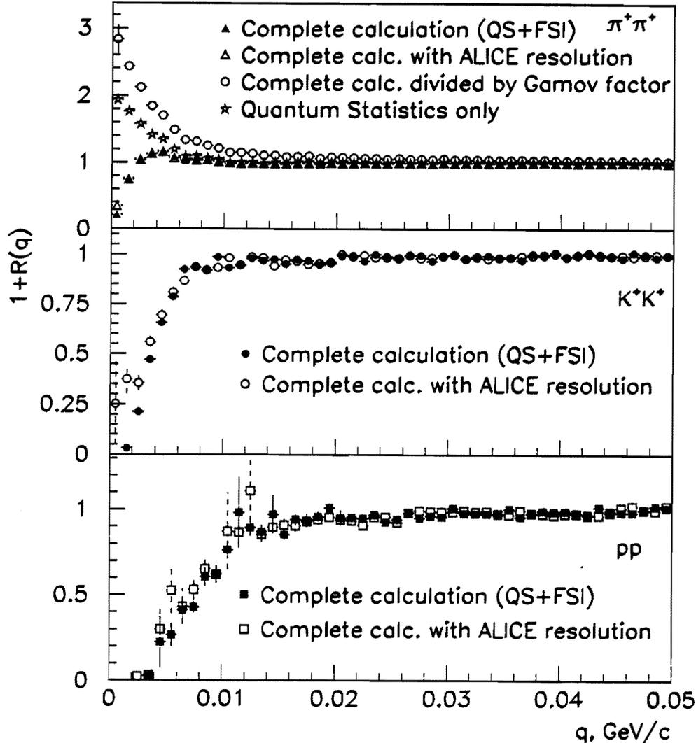
Fig. 17 Simulated correlation functions for two identical charged pions, kaons and protons without and with the effect of experimental resolution accounted for. The simulations were done using VENUS model with extended space-time freeze-out coordinates to set  $\langle r \rangle = 30 \text{ fm}$  and  $\langle t \rangle = 20 \text{ fm}/c$ . For two pions the Gamow corrected correlation function is compared with that including the effect of quantum statistic only.
