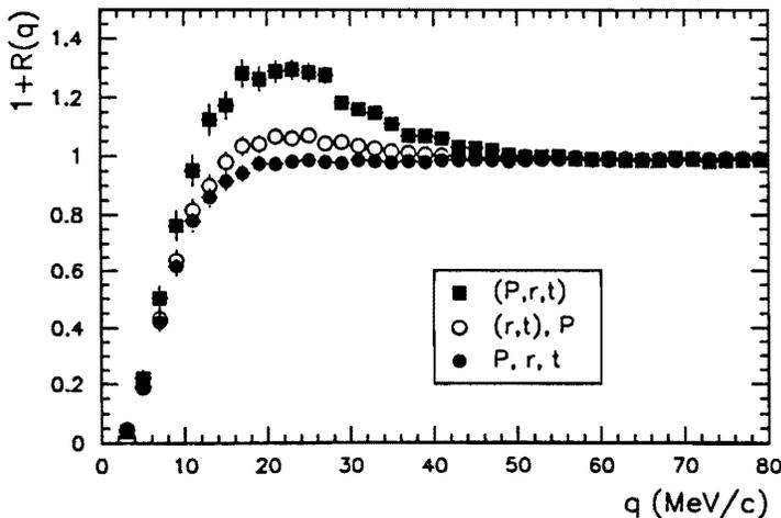
Fig. 10 Correlation function of two protons emitted in the reaction  $^{123}\text{Xe} + ^{48}\text{Ti}$  at 45 MeV/u predicted by QMD : with space-time coordinates and momenta of particles dynamically correlated (see Fig. 9) (squares) ; only space-time coordinates are correlated (open circles) ; space-time coordinates and momenta are decorrelated, i.e. taken from different events (solid circles).
