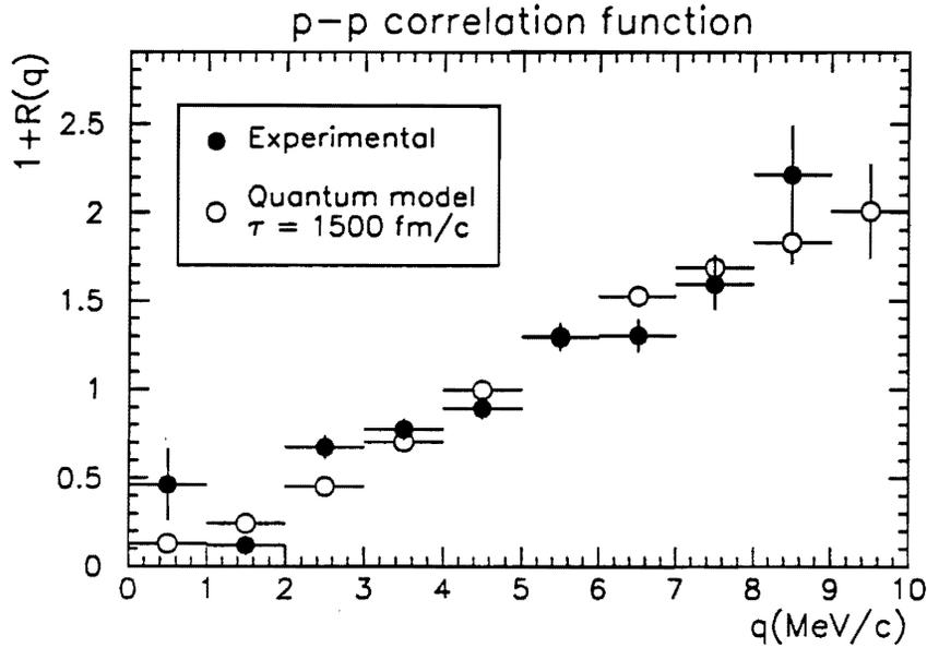
Fig.2 Two-proton correlation function measured in the region of very low relative momenta in the reaction  $^{133}\text{Xe} + ^{48}\text{Ti}$  at 45 MeV/u using the magnetic spectrometer SPEG at GANIL. Data are compared with calculation assuming the static source parametrization. Normalization was performed by setting equal areas of the correlated and uncorrelated spectra.
