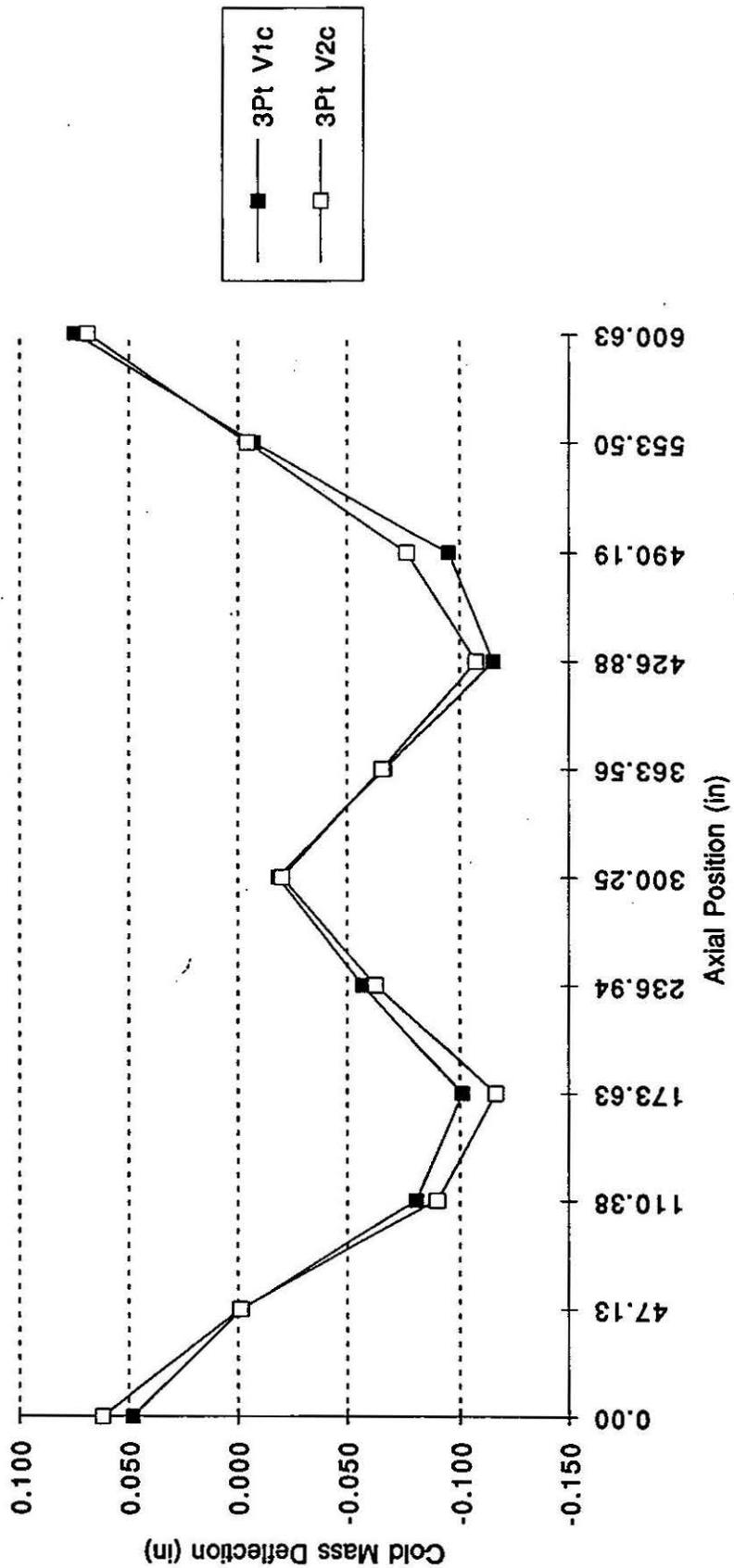
Table 3 and figure 3 show the data for the horizontal (designated with an 'H' in the headings) orientation of the yoke split in the same format as used in Table 2. The averages in both cases agree well, although the data from the horizontal orientation is much more scattered and unexpected, particularly at the east (0 inch) end of the magnet in the second trial. This data was repeatable, but remains unexplained.
